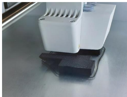
Figure 4.29: Printing stage of the new gripper fingertips. Reference: edited by Francesco Succurro
