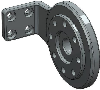
Figure 4.11: Gripper side interface plate. Reference: edited by Francesco Succurro
