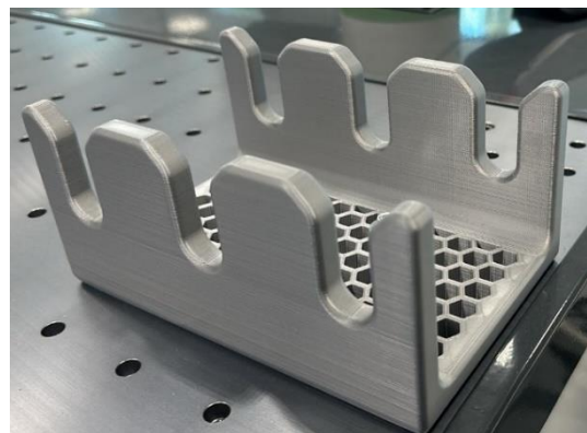
Figure 4.36: Printed boards tray. Reference: edited by Francesco Succurro
