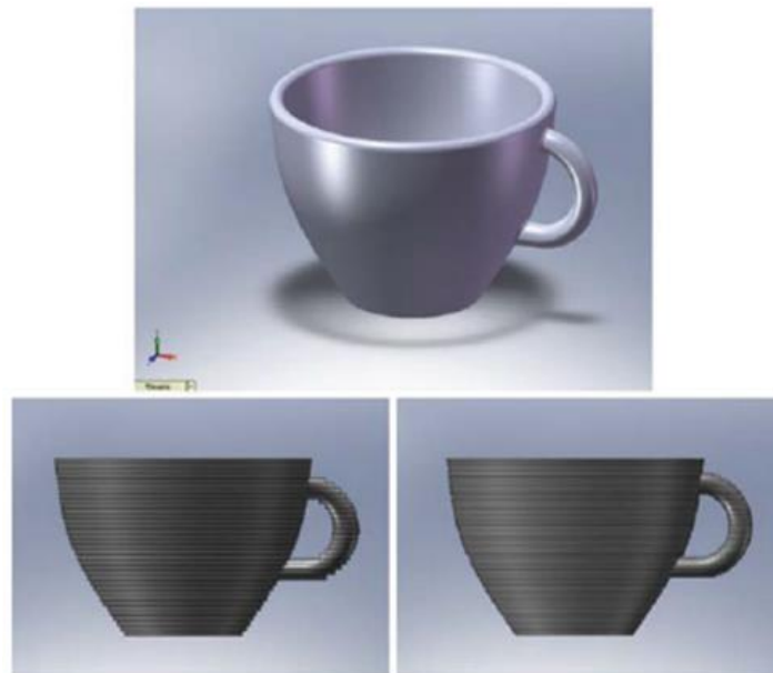
Figure 3.1: Images showing the CAD model of a component and the printing effects of using different layer thicknesses.
