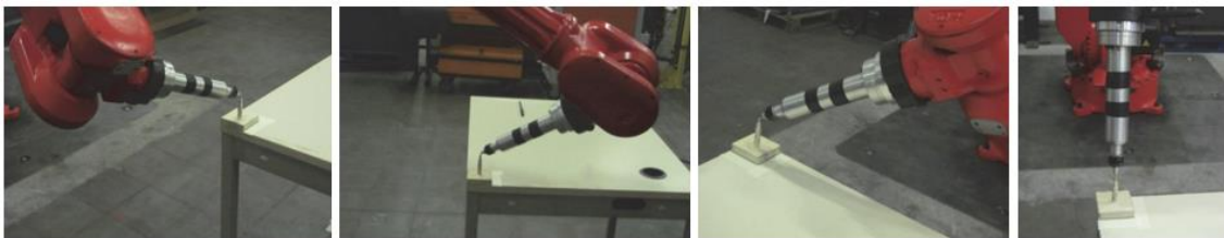
Figure 4.60: Four different orientations in which the tip of the Tool Master touches the tailstock. Reference: Fanuc Italia S.r.l.
