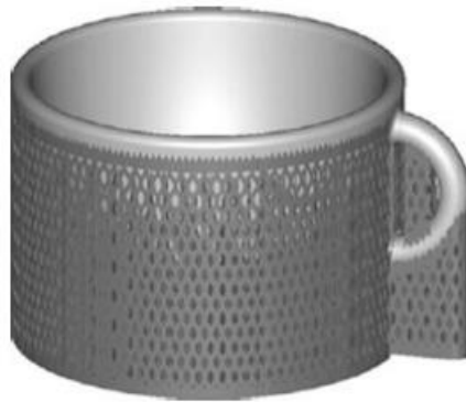
Figure 3.4: Supports generated for printing the component. Fonte: I. Gibson, D. Rosen and B. Stucker, Additive Manufacturing Technologies: 3D Printing, Rapid Prototyping, and Direct Digital
