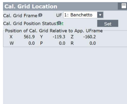
Figure 4.77: Calibration grid location. Reference: edited by Francesco Succurro
