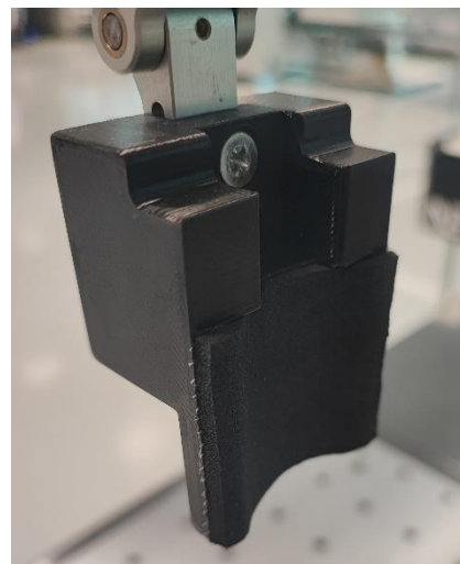
Figure 4.40: Detail of the grip fingertip coated with the adhesive neoprene. Reference: edited by Francesco Succurro
