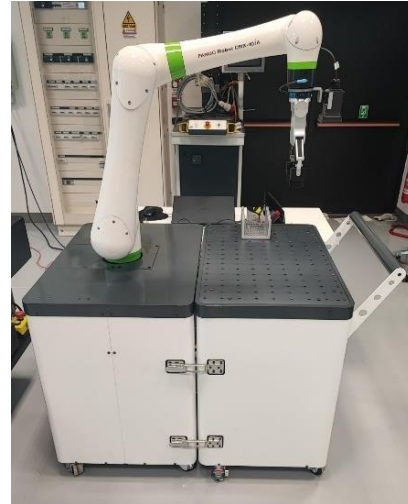
Figure 4.43: Collaborative robotics station. Reference: edited by Francesco Succuro
