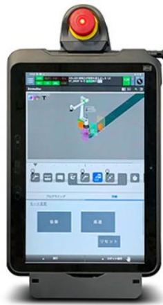
Figure 4.46: Tablet Teach Pendant. Reference: urlly.it/3yq2n
