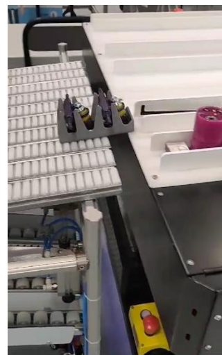
Figure 4.132: Push paddles with horizontal orientation. Reference: edited by Francesco Succurro
