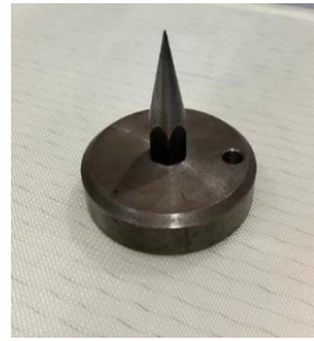
Figure 4.59: Tailstock of the Tool Master. Reference: edited by Francesco Succurro
