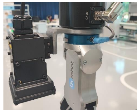
Figure 4.32: Interface plate mounted on the end effector of the robot. Reference: edited by Francesco Succurro
