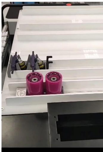
Figure 4.131: Push paddles with vertical orientation. Reference: edited by Francesco Succurro
