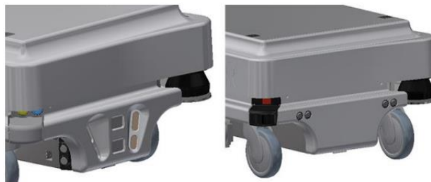
Figure 4.137: There are four ultrasonic sensors on the robot: two in the front (left) and two in the back (right). Reference: MiR 200 manual
