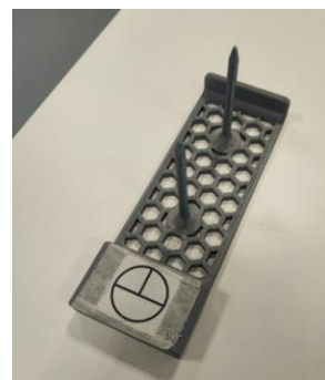
Figure 4.113: Wheels tray with the marker applied. Reference: edited by Francesco Succurro
