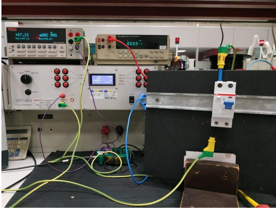
Figure 15: Setup test measuring the tripping current on a differential switch with a sensitivity of 10 mA. Shown are the Keithley 2001 in the top left, the Hytron in the bottom. All instruments are connected in series to the switch under test, which receives the fault current via pole R. The Hytron is set in AC ramp mode, so that it generates a sine wave of amplitude equal to the sensitivity of the instrument. (Di Pippo)
