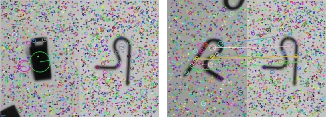
*Figure 6.8: matching result on wrong-posed pieces. The target piece on the left (5<sup>th</sup> in the full image) has no match pairs, while the one on the right (the 9<sup>th</sup>) presents match pairs even if its pose is incorrect*
