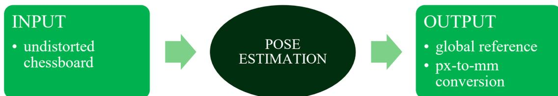
One main assumption must be considered before starting: to simplify computations, the camera XY plane is assumed to be parallel to the world XY plane, or also the coordinate axis Z, perpendicular to the image plane, is considered coincident with the Z axis of the camera. This is true only if the camera is correctly placed above the platform, with very small rotations around the X and Y axes.
