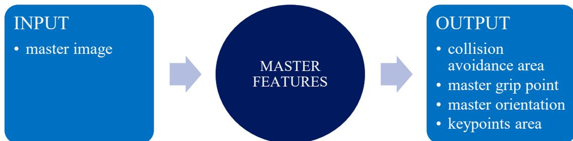
As for the master thresholding parameters and the master blob area, all these values must be set only the first time a new kind of pieces is considered.
