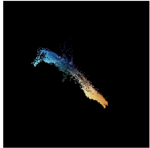
Figure 3.14: Vectorscope of the raw image
