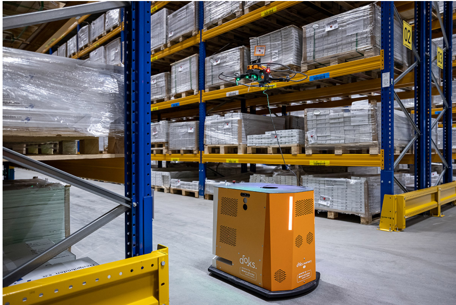
Figure 2.9: AMR that supplies power to a drone with a cable
