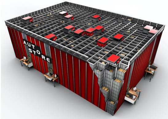
Figure 2.3: Autostore: an automated storage and retrieval system
