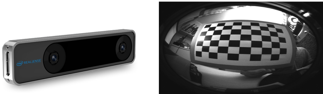
Figure 3.8: Example of a camera with fisheye lenses: T65, also used in our tests. The second picture is an example of type of picture it can take.
