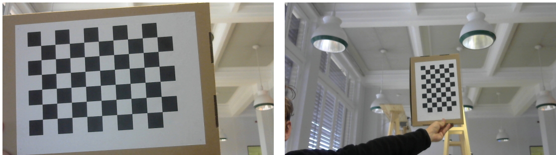
Figure 4.11: Example of calibration chessboard image acquisition
