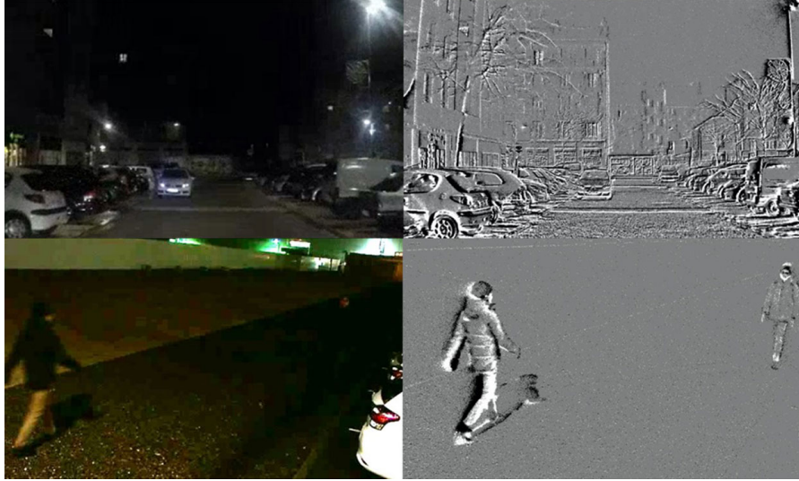
Figure 3.10: Event-based camera output example
