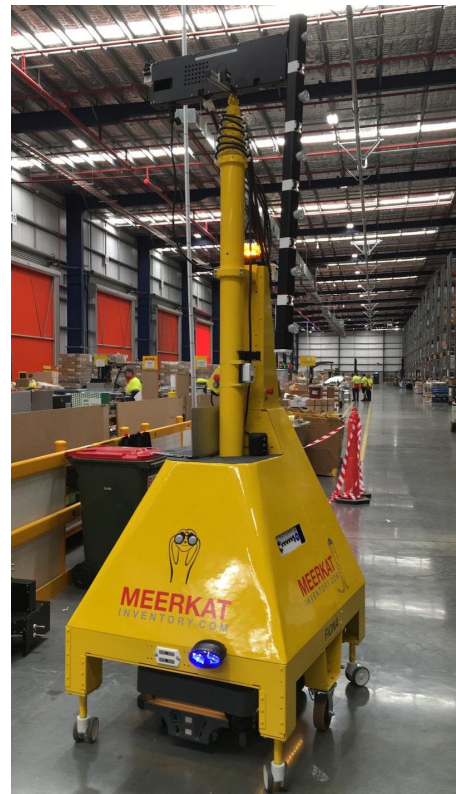
Figure 2.10: Example of AMR with a telescopic pole and a camera
