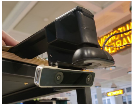
Figure 4.3: Photo of the T265 and Logitech webcam holder
