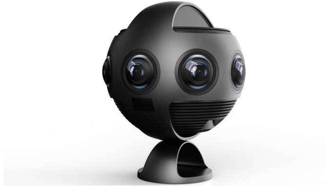
Figure 3.6: Example of an omnidirectional, 360° camera
