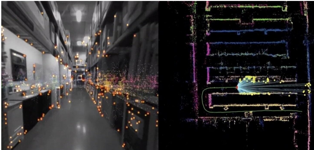
Figure 2.5: VIO (Visual Inertial Odometry) example
