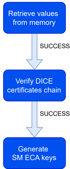
Figure 7.4. DICE architecture’s process during SM initialization.
