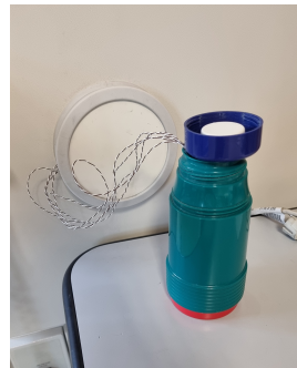
Figure 4.6: Dewar used to create the 0^{\circ}\text{C} reference
