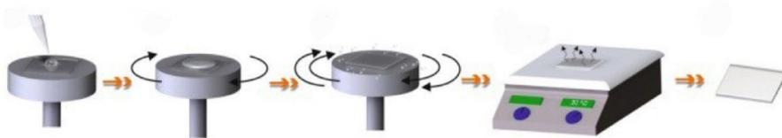
**Figure 2.7:** Schematic representation of the preparation of  $\beta$ -PVDF by spin coating. With the help of a syringe the PVDF solution is deposited on the substrate located on the rotary disk of the spin coater; proceed the deposition step at rotational velocity of 4000 rpm for 30 s; place the film onto a hot plate at 70 °C; and the PVDF film is ready.<sup>(19)</sup>
