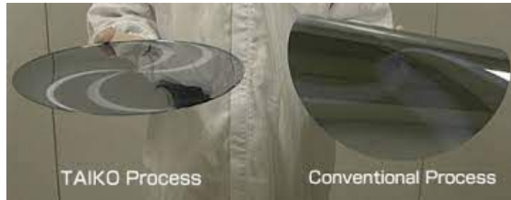
Figure 5.9: On the right the thinning of the silicon wafer with the conventional back grinding technique and on the left the thinning of the silicon wafer with the Taiko process [49]
