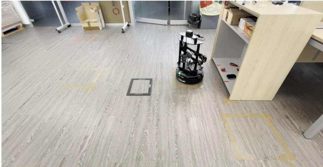
**Figure 8.16:** After the planner has found a suitable trajectory, the mobile base final pose is extracted and assigned to the Base Handler node. As a result, the mobile base is moved to a different position with respect to the one where the object detection pipeline started.
