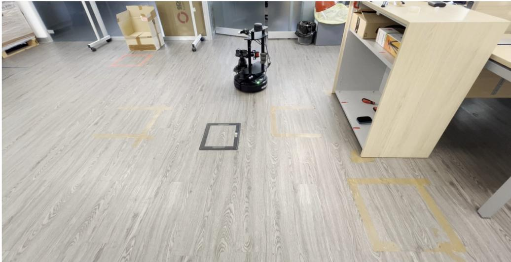
**Figure 8.20:** After the success of the grasp action, the mobile manipulator approaches the depot location to release the object.
