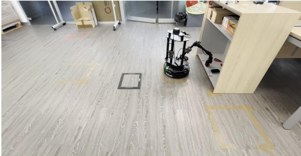
**Figure 8.18:** Once the pre-grasp pose is reached, the Communication Manager requests to the Arm Handler a plan to reach the grasp pose. When in this pose, the gripper is closed to grasp the object.
