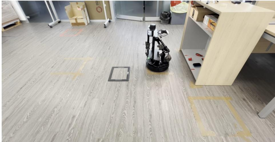
**Figure 8.14:** After a request is received, the searching phase starts, and the mobile manipulator goes to the first known location. Here the Object detection phase starts, and if the requested item is present in the current location, the LoCoBot Extended Planner node is called to find a suitable trajectory to reach the pre-grasp pose.
