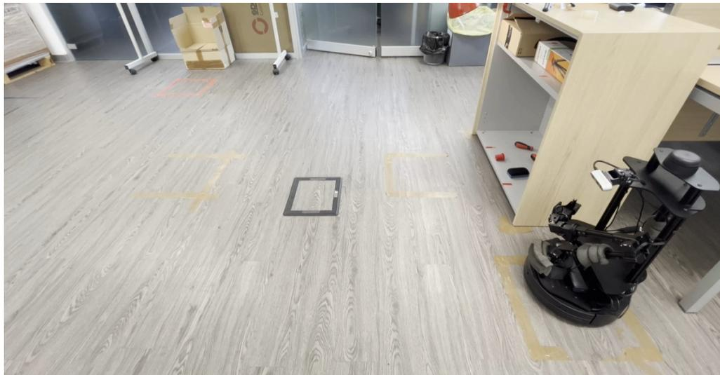
**Figure 8.13:** The LoCoBot always starts from the Home Position, right next to the desk of the human it is assisting. It is possible to notice how the arm is retracted in order to not exceed the collision shape of the mobile base, thus not generating unexpected collisions.
