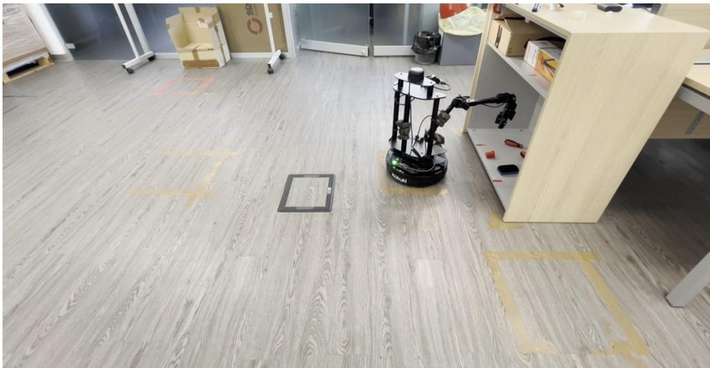
**Figure 8.17:** After the mobile base has reached the correct position, the trajectory computed for the arm is executed and the pre-grasp pose is reached. In this figure, it is possible to see the pre-grasp pose right above the object and the gripper open.
