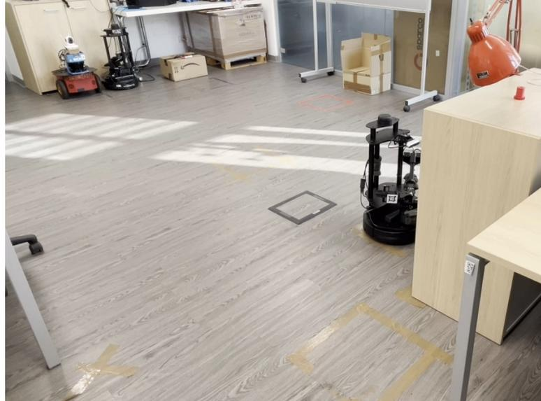
**Figure 8.8:** The LoCoBot reaches the target location. Here the object detection task is executed, involving the Grasping Point Generator node to compute the predictions using the trained YOLOv5 network.
