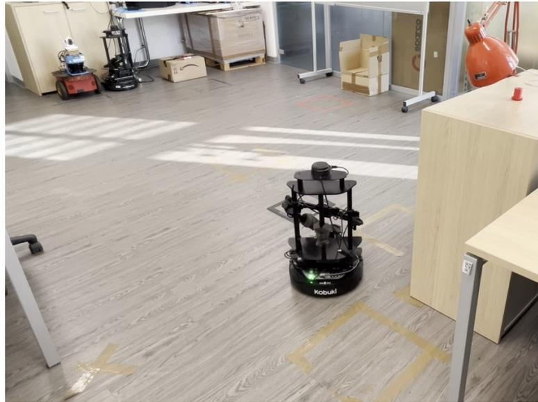
**Figure 8.7:** After the Communication Manager receives a request, it extracts the first known location where it is possible to find the requested item. In this case, the first place is the Dataset Location, hence its coordinates are extracted and the control is demanded by the Base Handler that computes a path to reach the target.
