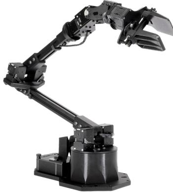
**Figure 4.2:** WidowX 250-6DOF Robot Arm used on the LoCoBot WX250s.
