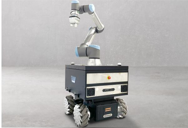
**Figure 1.5:** Example of a wheeled mobile manipulator [9].
