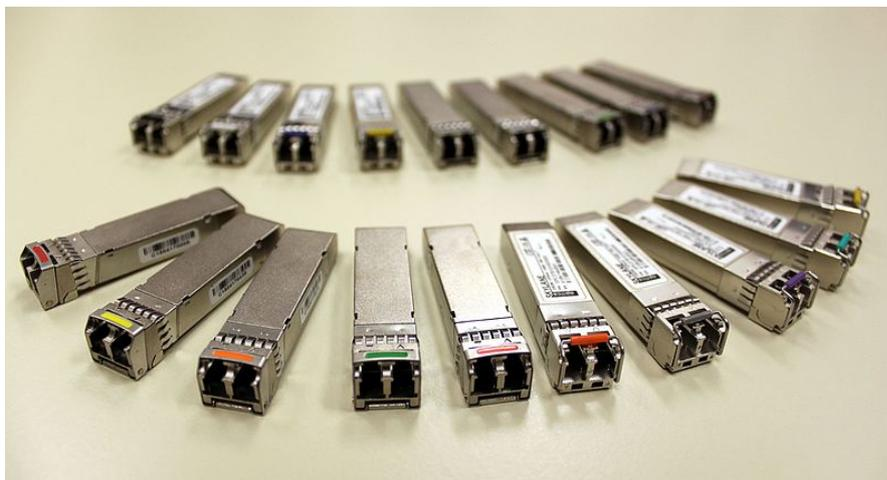
**Figure 2.1:** Picture showing standard transceivers. Source: [4]
