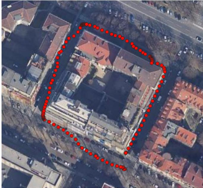
Figure 5.36. GNSS trace - short round path test with heading threshold set to 4 degrees
