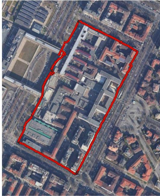
Figure 5.45. GNSS trace - long round path test with heading threshold set to 10 degrees
