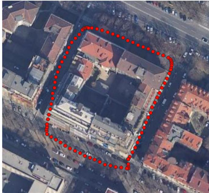
Figure 5.39. GNSS trace - short round path test with heading threshold set to 10 degrees
