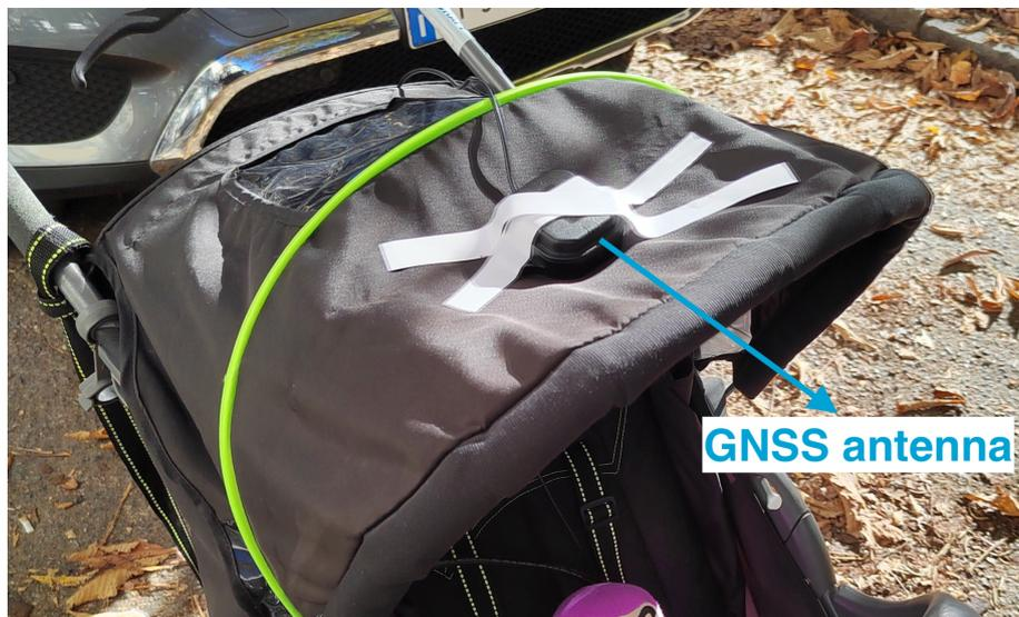
Figure 5.22. GNSS antenna
