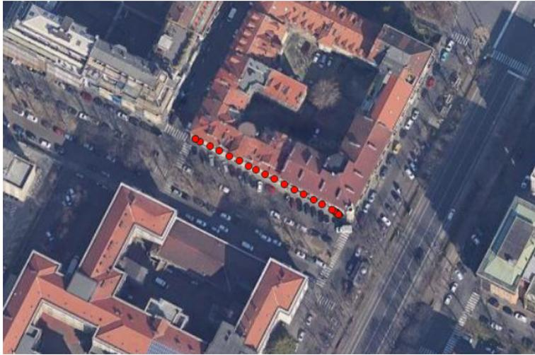
Figure 5.30. GNSS trace - straight path test with heading threshold set to 4 degrees
