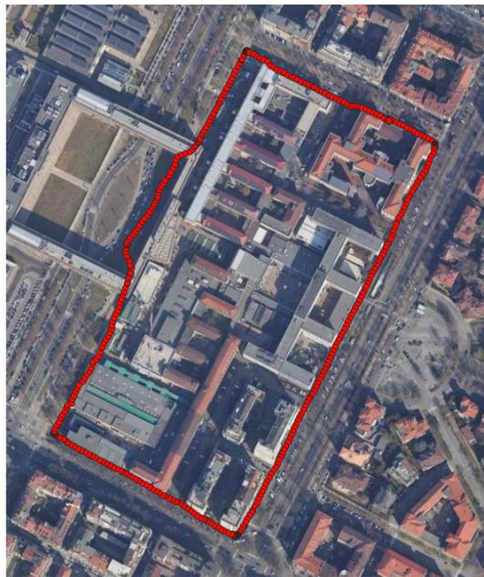
Figure 5.42. GNSS trace - long round path test with heading threshold set to 4 degrees
