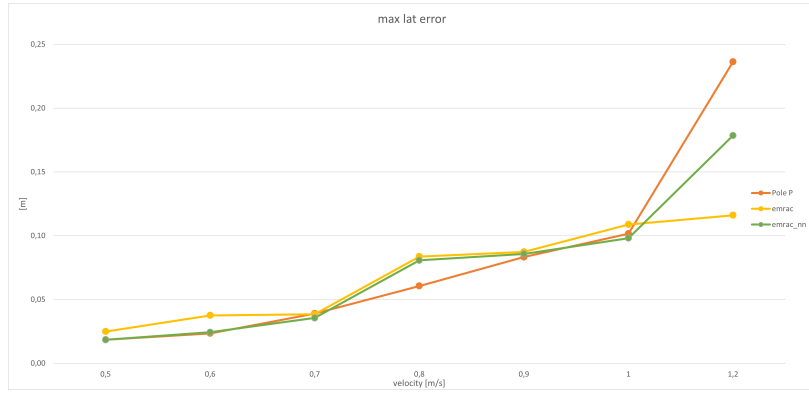
Figure C.15: Maximum lateral displacement error, 2nd lap
