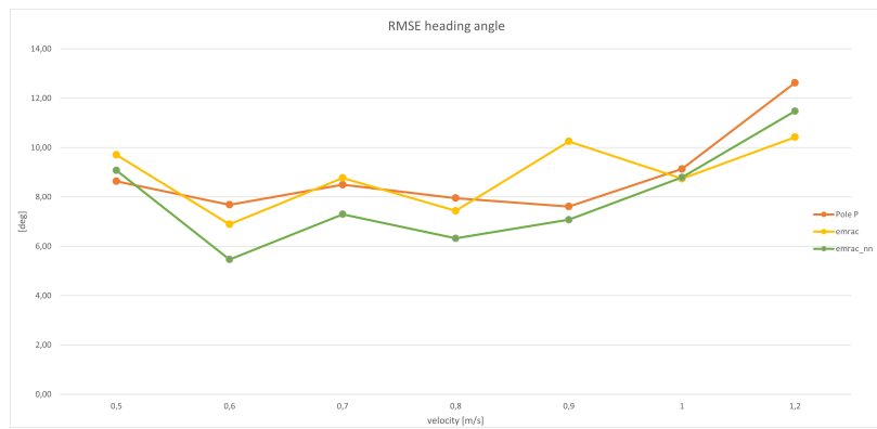
Figure C.18: RMSE heading angle error, 2nd lap
