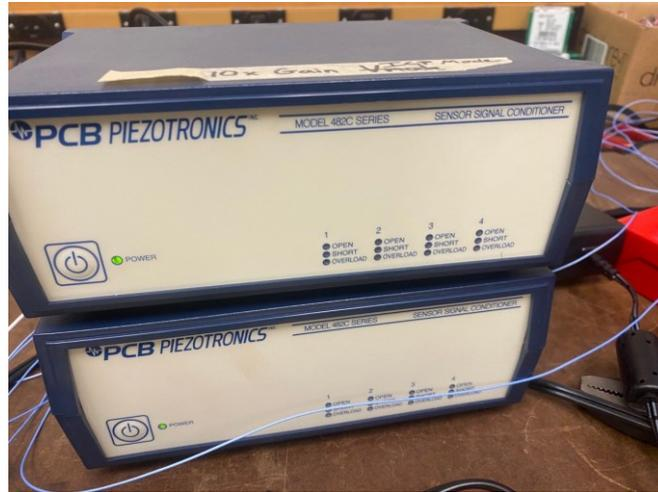
Figure 3.5 PCB Piezotronics model 282C series sensor signal conditioners
