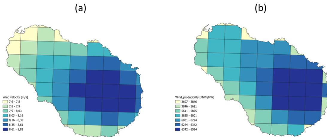
Figure 26 - Wind mean velocity (a) and producibility (b) for the Pantelleria Island.
