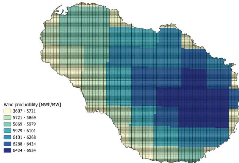
Figure 27 - wind producibility @100m map of Pantelleria with a finer grid
