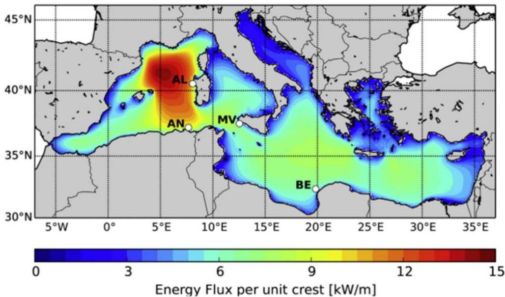
*Figure 18 – Mean wave energy flux from 1979 to 2013 [79]*
