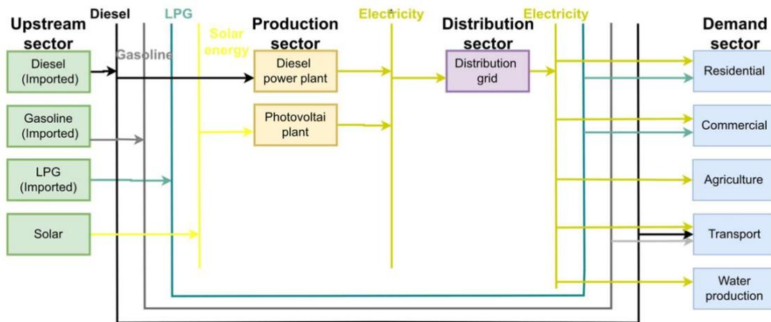
Figure 15 – Pantelleria electricity sector representation [67]
