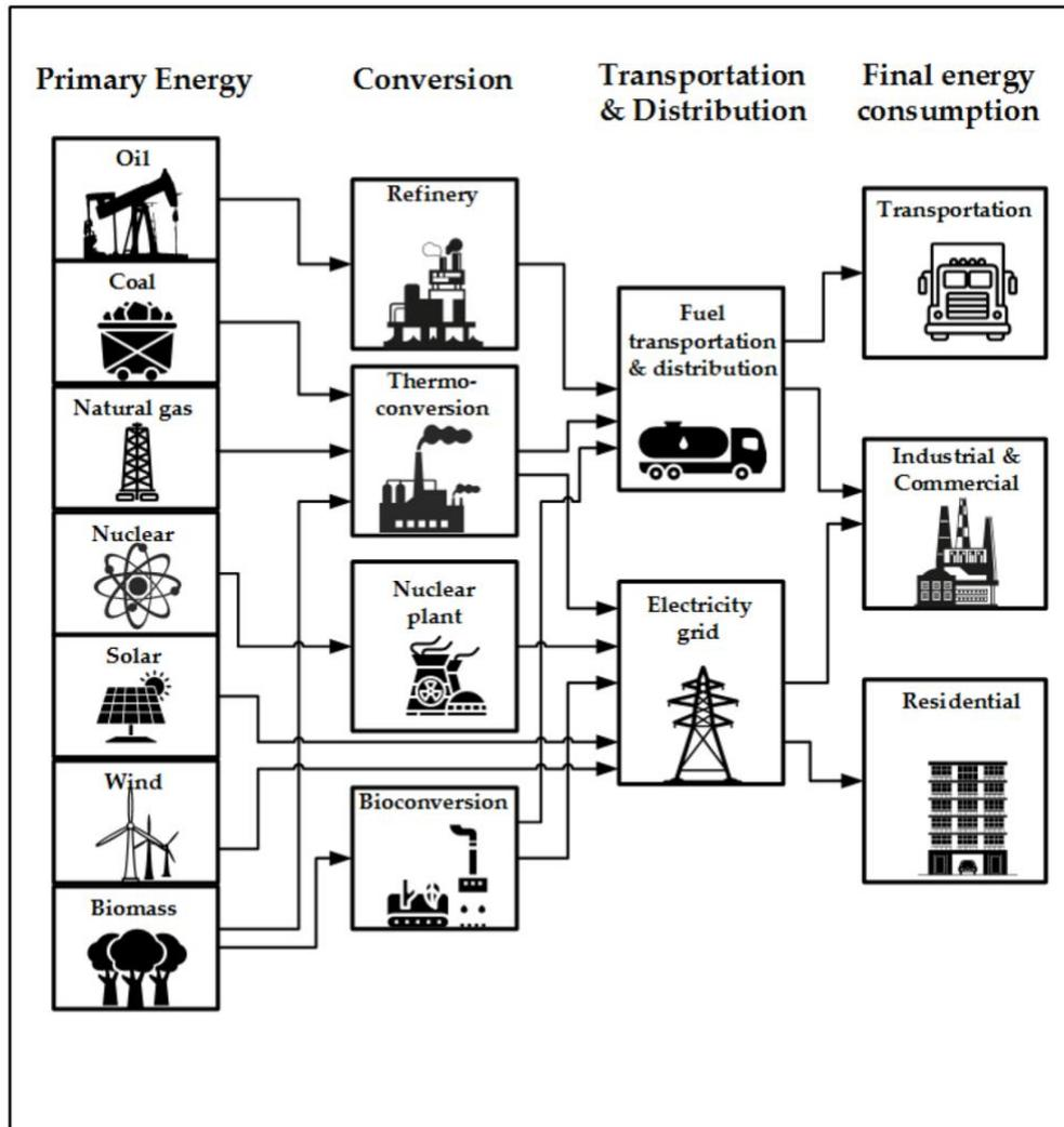
Figure 6 - Energy system showing the flow of energy from primary energy supply to final energy consumption [30]
