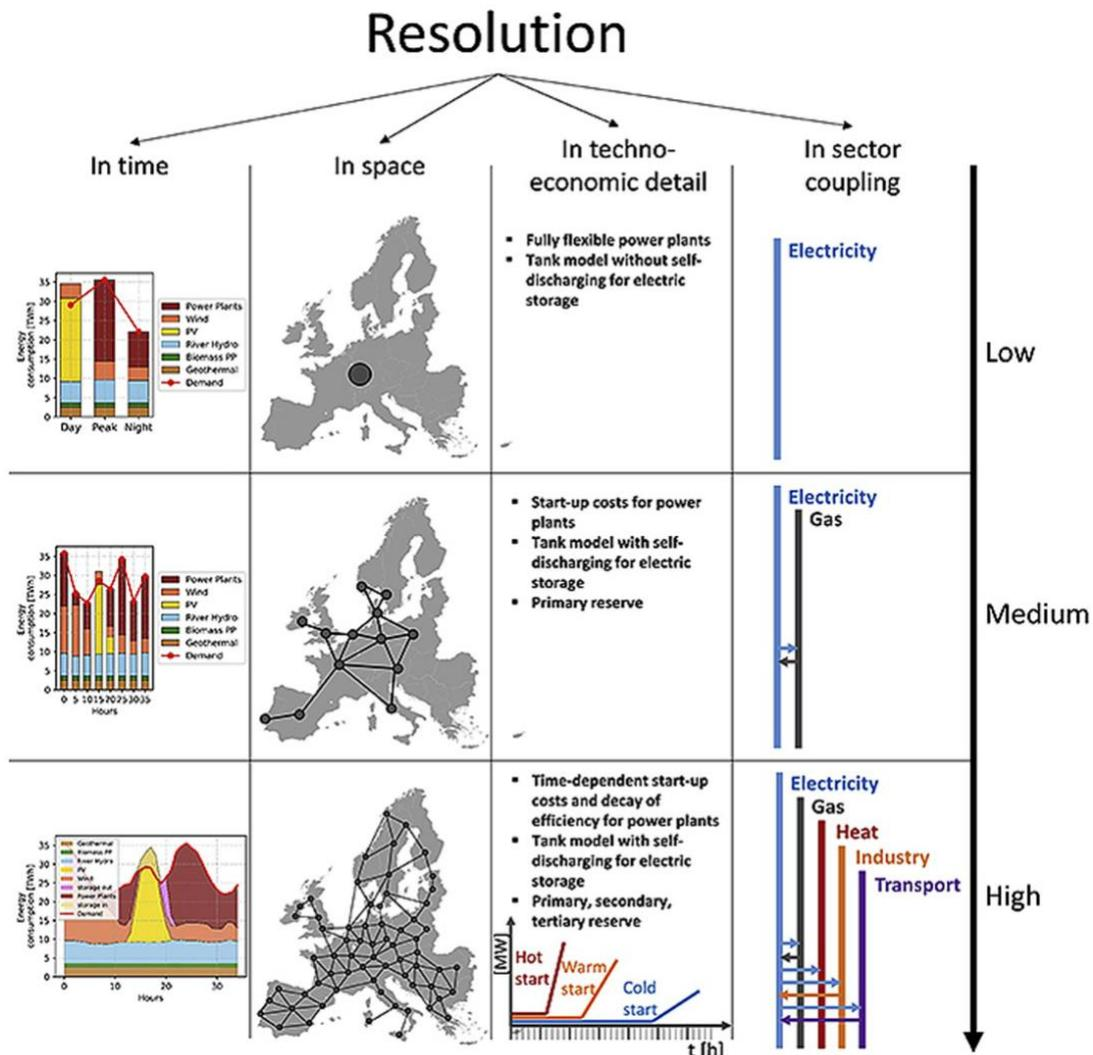
Figure 7 - Possible resolutions of bottom-up energy system model [34]
