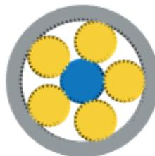
**Figure 5.6:** 2-D configuration of stage 1 from KISSsoft
