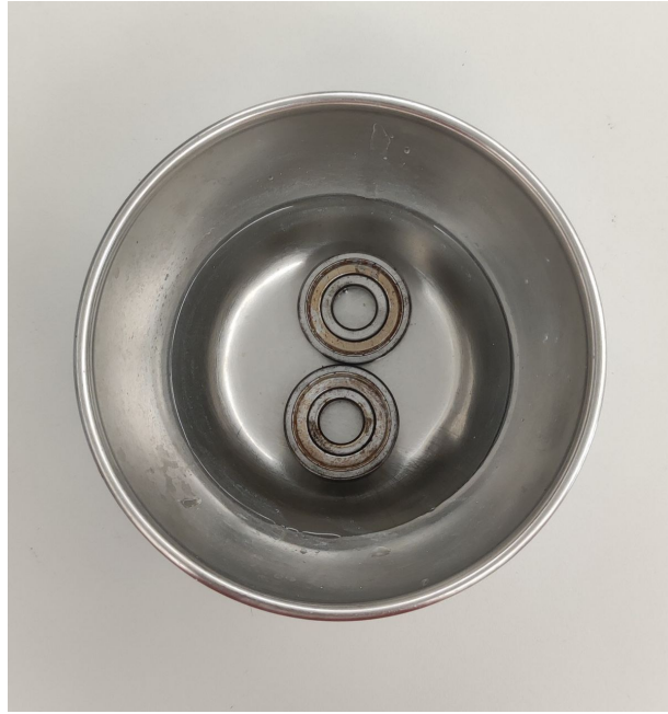
Figure 3.2: Grease removal process from the bearings
