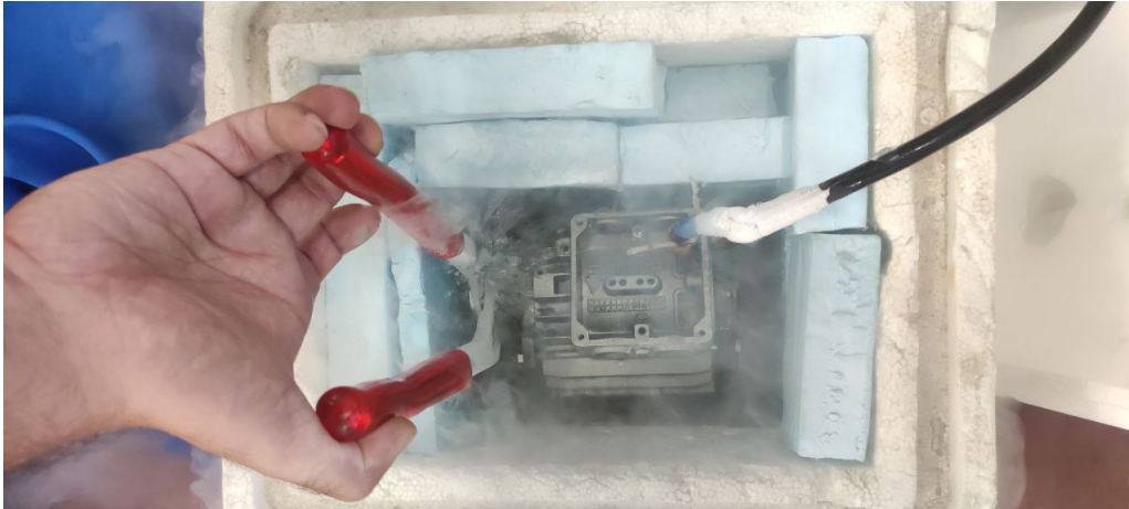
Figure 3.8: Locked rotor test setup in cryogenic conditions
