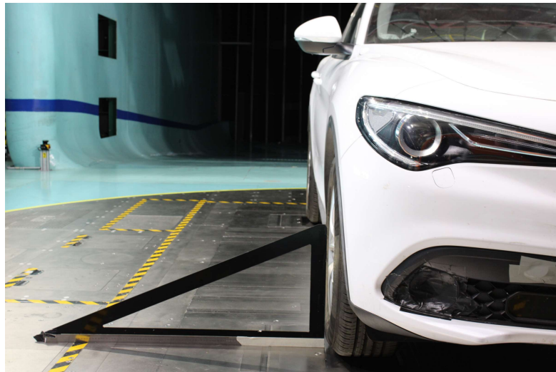
Figure 5.24: Tangent wheel position wrt WSU
