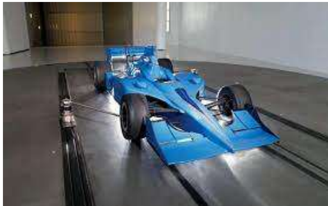
Figure 4.1: Single belt moving ground set-up
