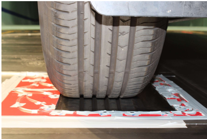
Figure 5.26: Belt pressure field sensors
