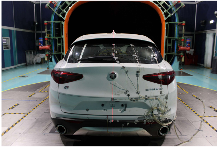
Figure 5.25: Rear pressure field sensors
