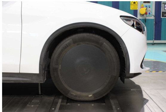
Figure 5.21: Carbon wheel cover
