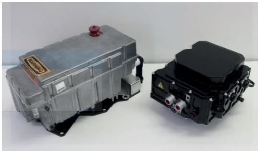
(a) Si IGBT based 200kW inverter on the left and SiC MOSFET based 220 kW inverter on the right
