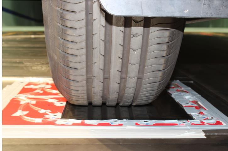
Figure 6.4: Position sensors around the wheel
