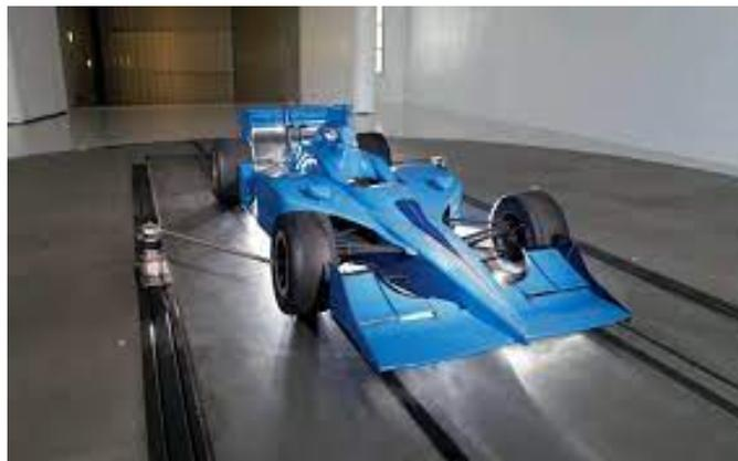
**Figure 4.1:** Single belt moving ground set-up
