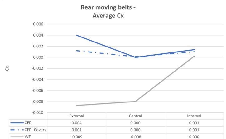
**Figure 6.15:** Comparison CFD and WT Cx average during reae moving belts with covered wheels
