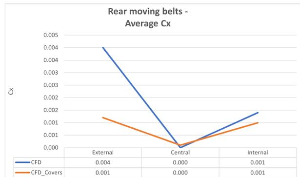
**Figure 5.31:** Average  $C_x$  during rear moving belts with covered wheels
