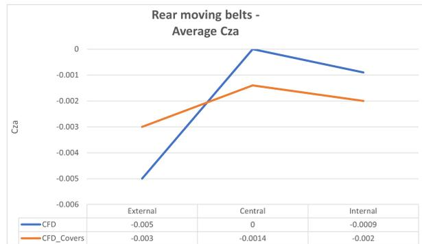
**Figure 5.32:** Average Cza during rear moving belts with covered wheels
