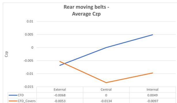
**Figure 5.33:** Average Czp during rear moving belts with covered wheels
