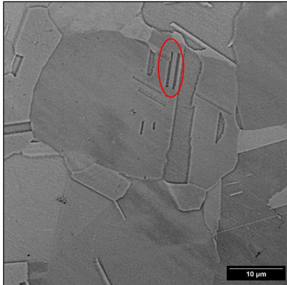
**FIGURA 42: MICROGRAFIA SEM DEL CAMPIONE 99, IN625, SOL AD INGRANDIMENTO 5000X CON MESSA IN RISALTO DEI BORDI DI GEMINATO**
