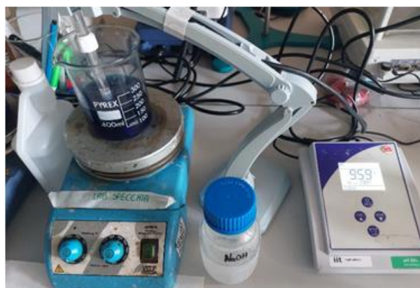
Figure 23: Setup for pH measurements
