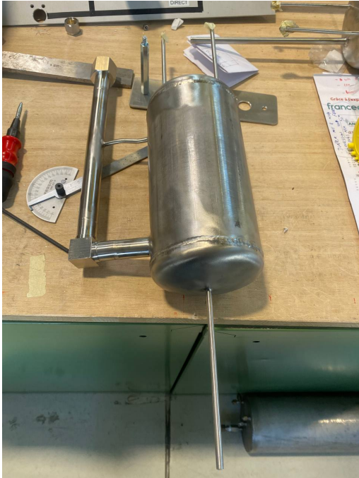
Fig. 4.39 Picture of the Reboiler Drum.
