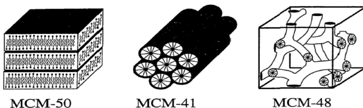
Figure 12. Schematic refiguration of the materials of the M41S family, MCM-50 (layered), MCM-41 (hexagonal) and MCM-48 (Cubic). [41]
