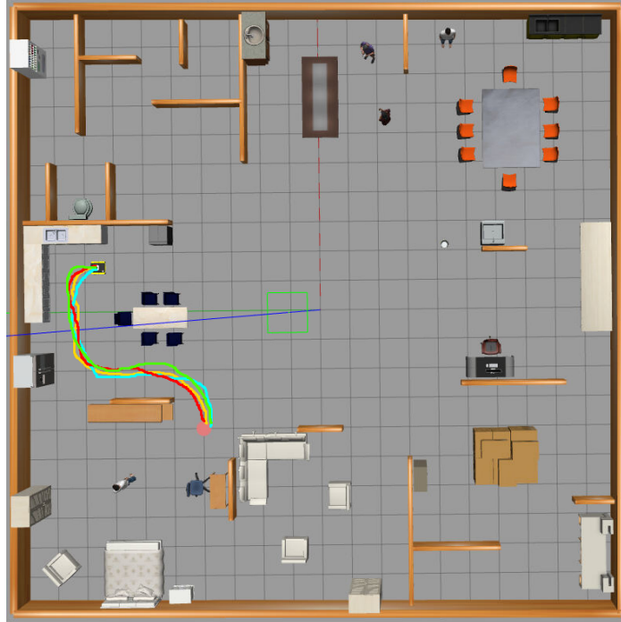
Figure 7.5: Trajectories from: [1.5, 7.5, -1.57] to [-4, 4] . Yellow: IQL, red: EDAC, light blue: BCQ, green: CQL
