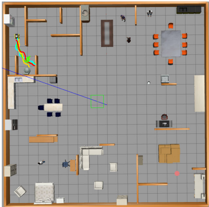
Figure 7.7: Trajectories from: [7, 9, 3.14] to [-7, 7] . Yellow: IQL, red: EDAC, light blue: BCQ, green: CQL
