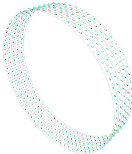
Figure 2-14 illustration of one ring lining (SAP2000)
