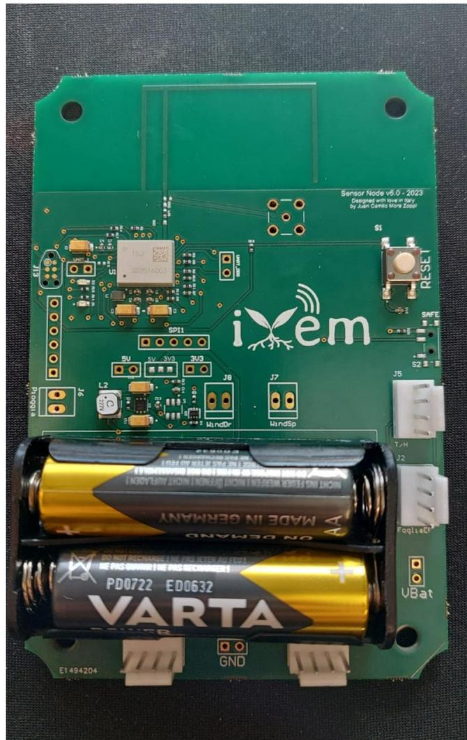
Figure 7.7: Sensor node PCB after manufacturing and assembly
