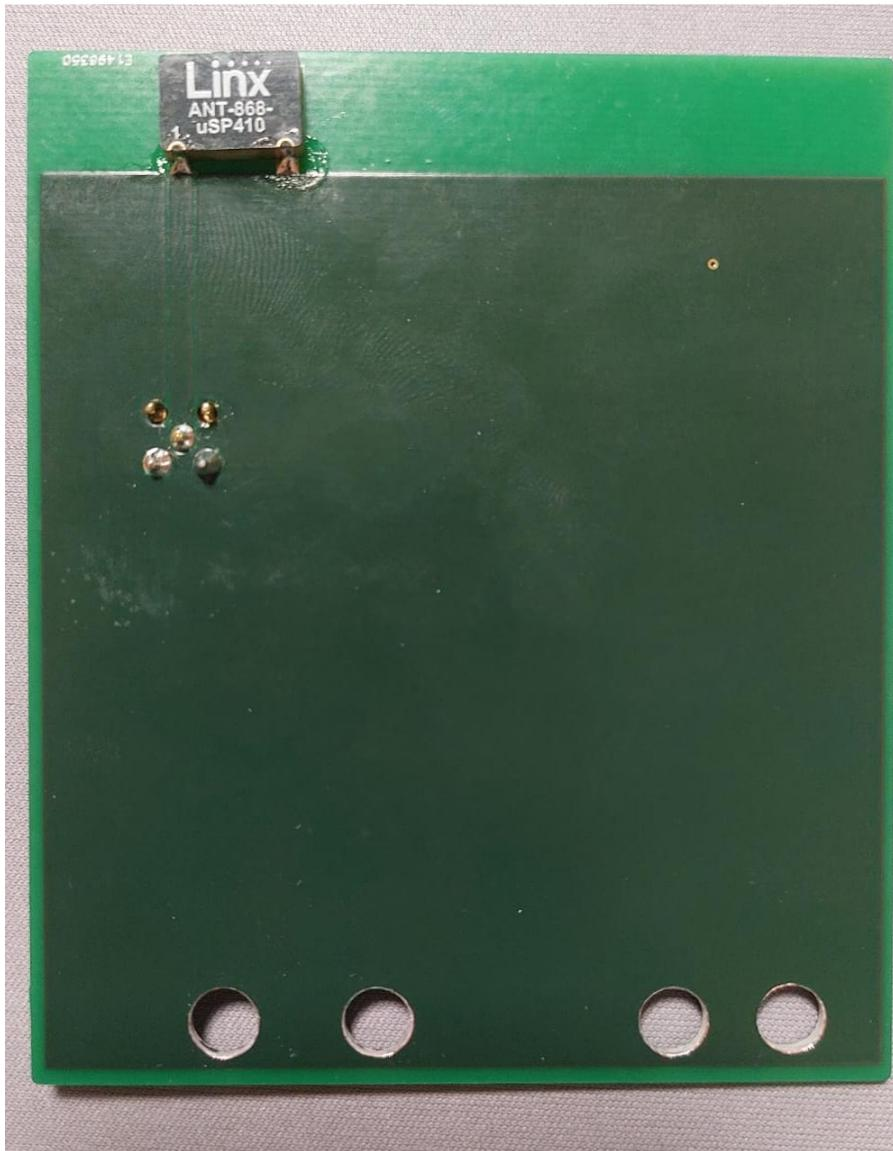
**Figure 5.27:** PCB Design: Chip Antenna
