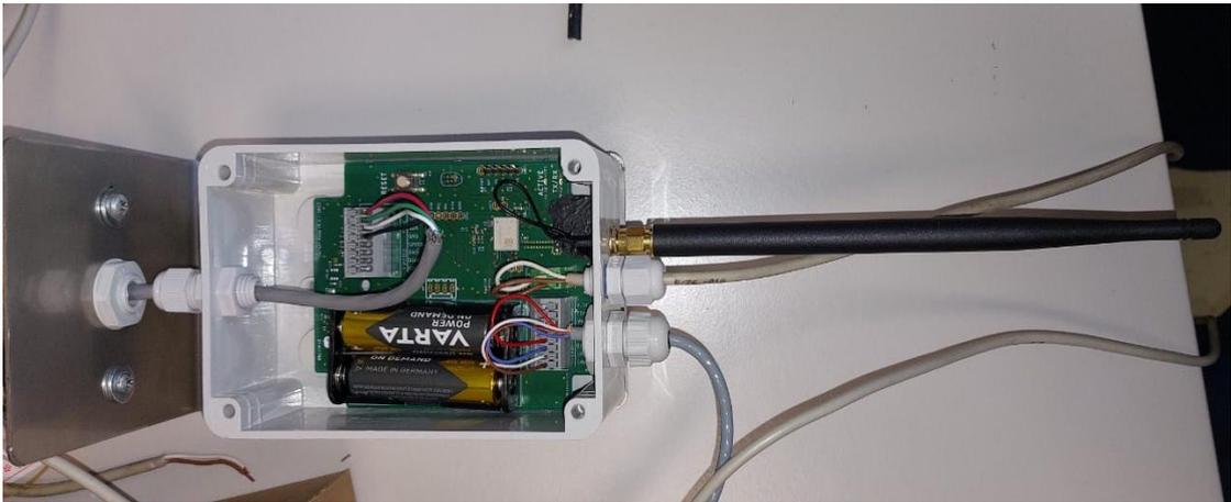
**Figure 1.2:** Current generation of sensor node PCB
