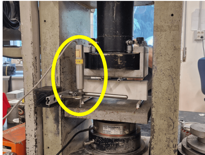
Figure 16: Measuring device and deflection device placed in a plate under the actual specimen.
