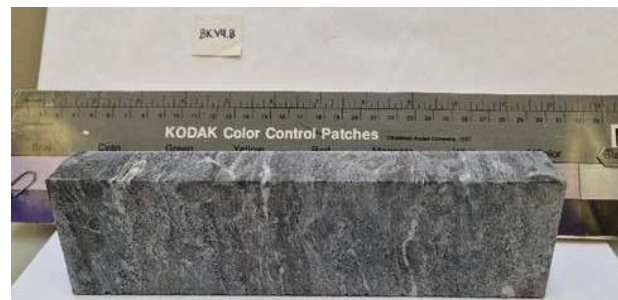
Figure 37: Prismatic rock specimen for type black.
