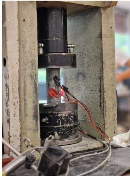
Figure 8: Loading device uniaxial compressive test.
