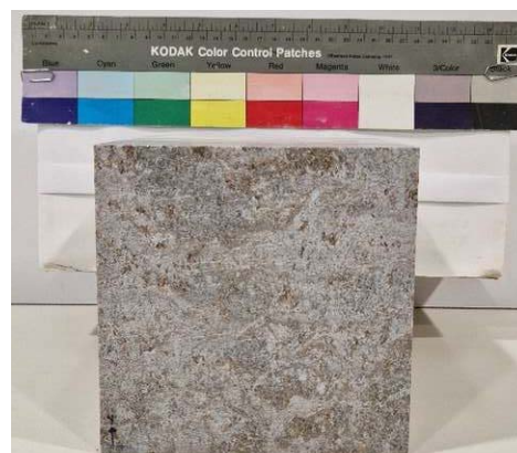
Figure 39: Cubic specimen for type brown.
