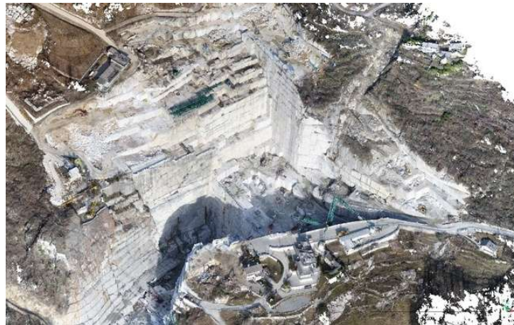
Figure 27: Reconstruction of the quarry by photos taken by an UAV and processed.
