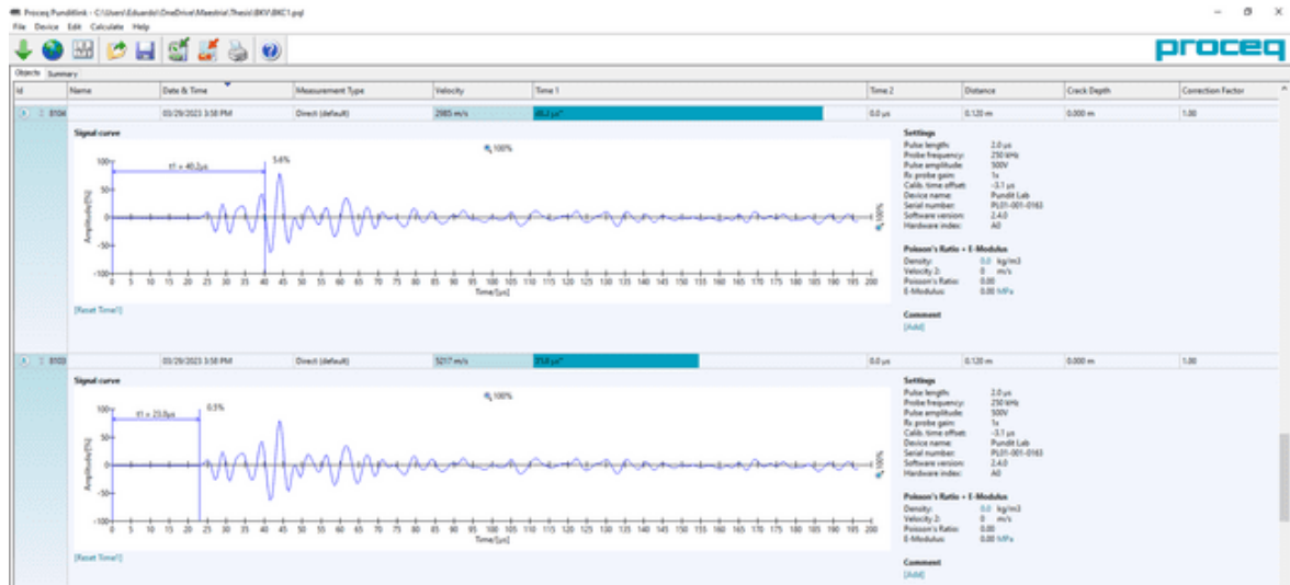
Figure 6: Example of picking the shear and compression waves in the software.
