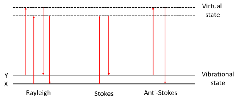
Figure 2.15 Schematic of the Rayleigh and Raman processes.
