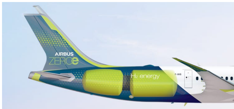
Figure 1.5: Airbus Zeroe turbofan - positioning hydrogen tank in fuselage [21]
