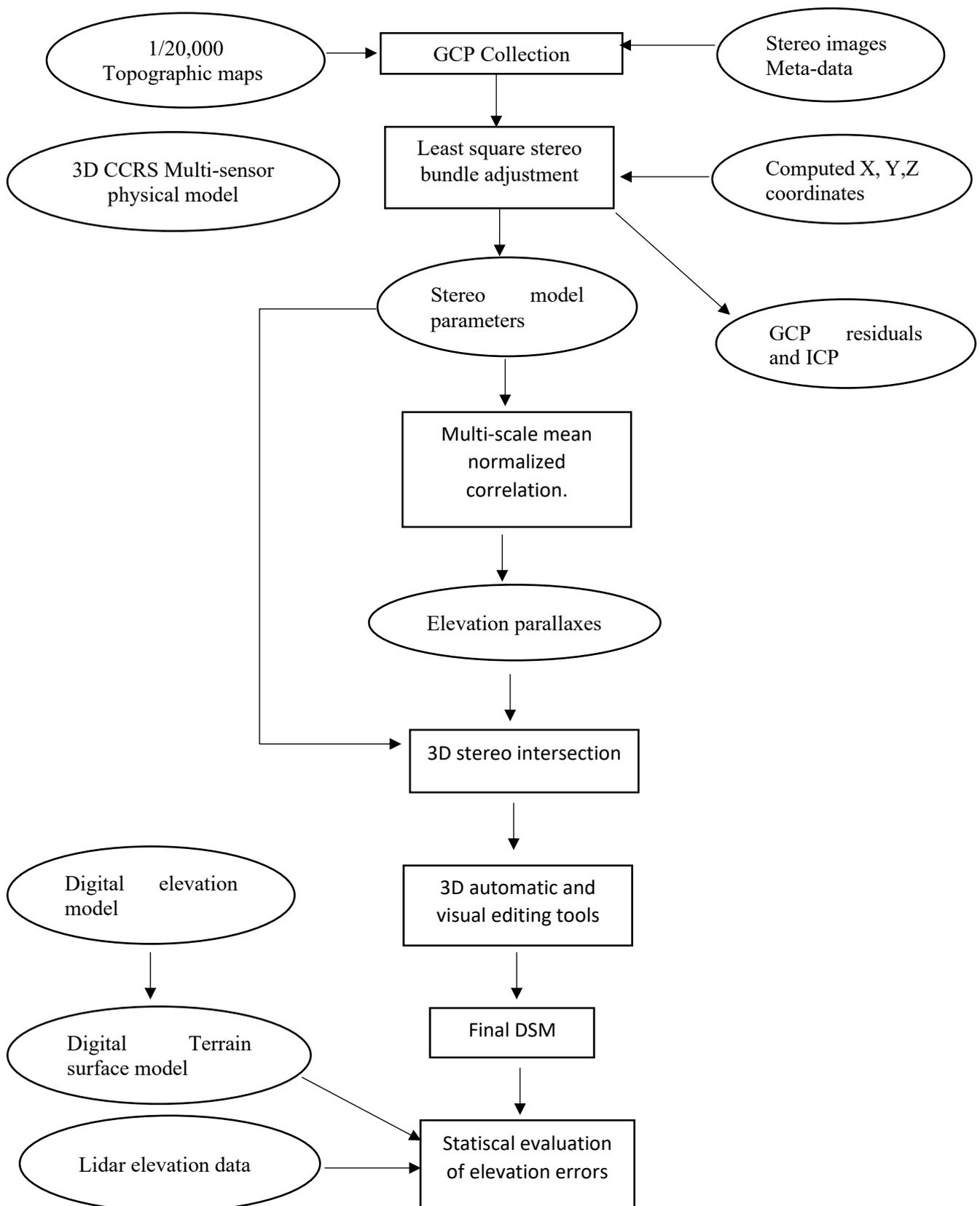
**Figure 5.3** Flow chart of the Processing steps for the generation of DEMs from stereo-images and their evaluation with LiDAR data.
