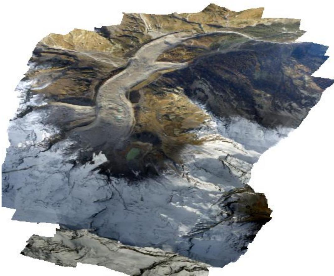
**Figure 6.2** Orthophoto of belvedere glacier of 15cm resolution generated by Politecnico di Torino glaciology lab in 2019 using Drones and UAV and Photogrammetry techniques and Lidar.
