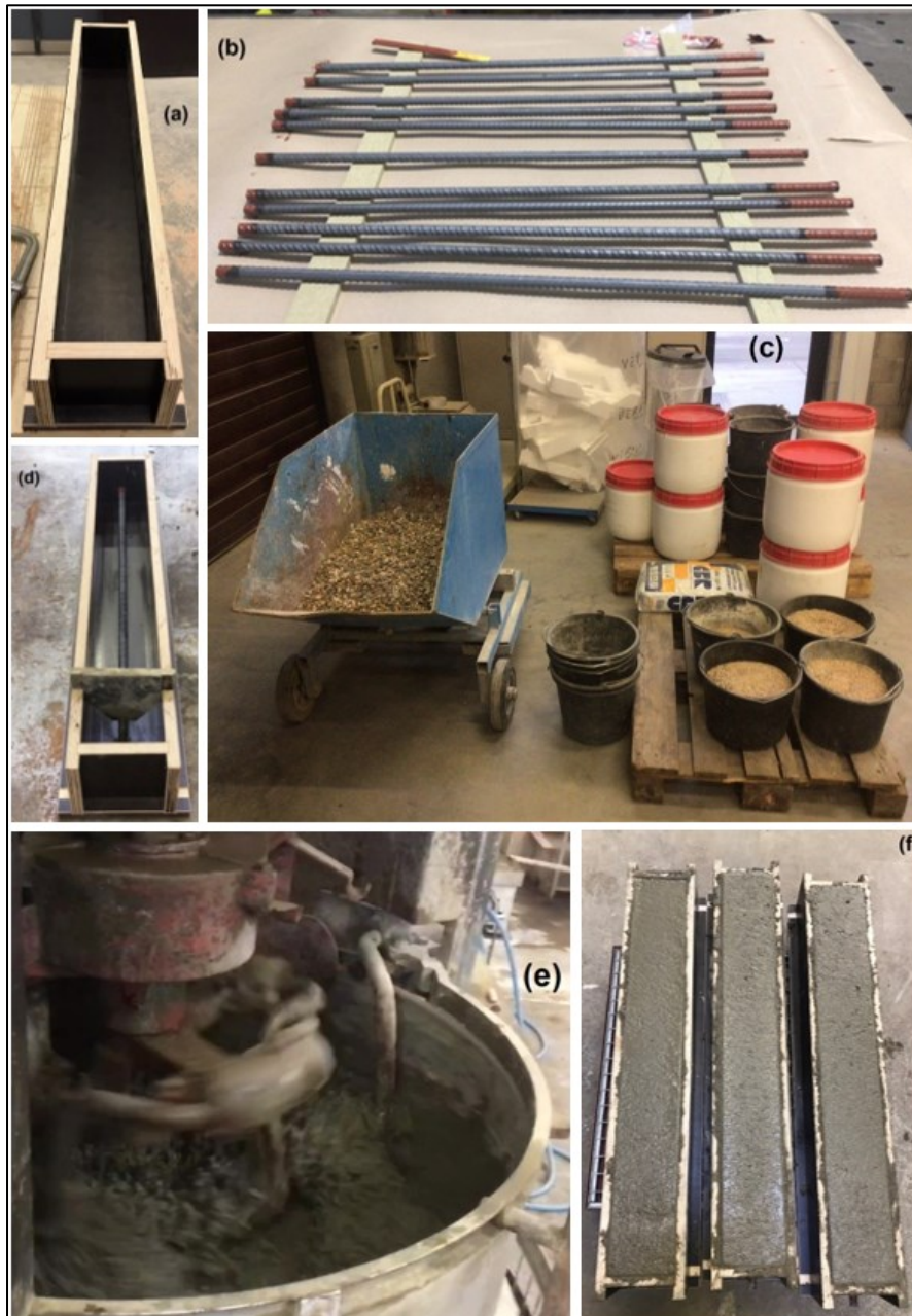
Figure 20: Casting process photographs: (a) Mould; (b) Rebar; (c) Concrete mixture preparation; (d) Rebar placed on the mould; (e) Concrete mixing; (f) RC specimens
