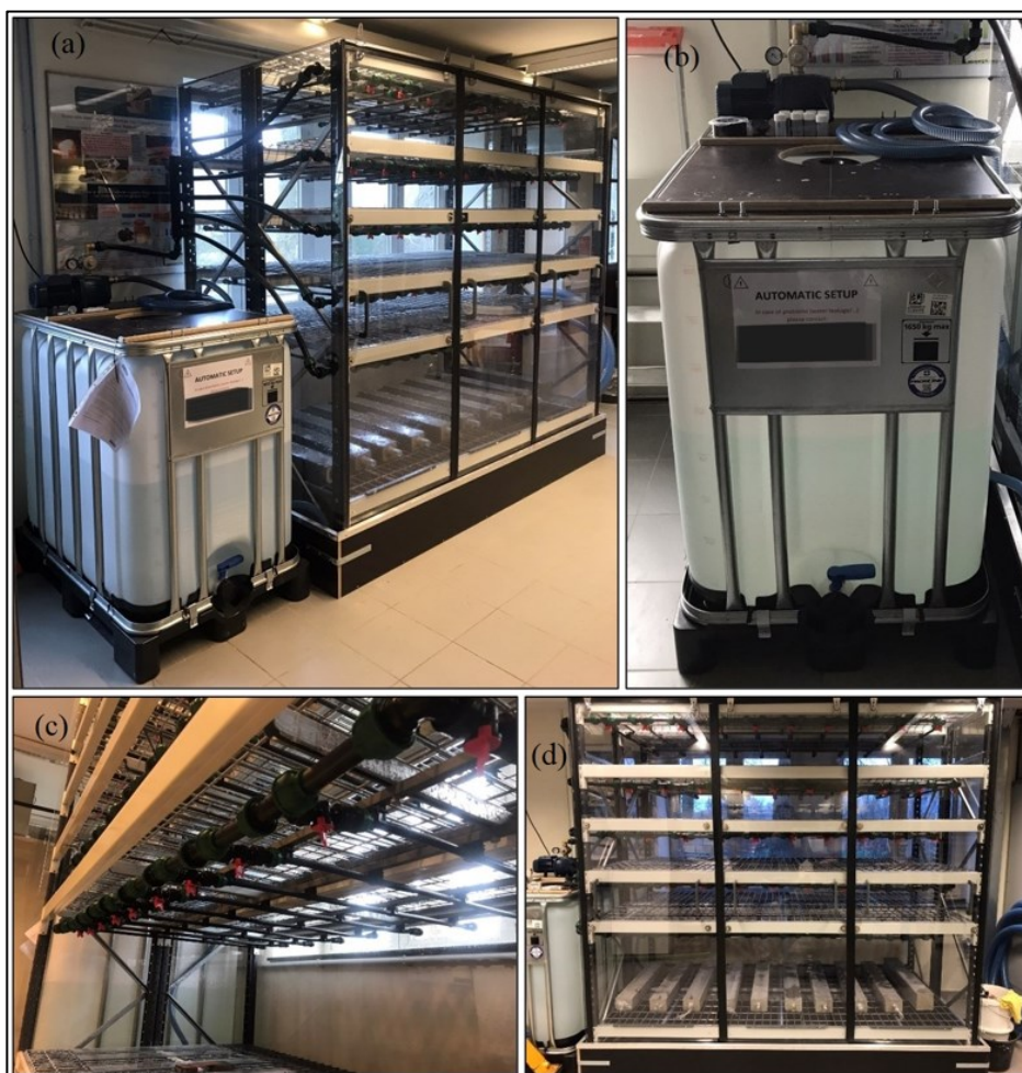
Figure 35: Natural corrosion setup: (a) Entire corrosion setup, (b) Tank, (c) Tubes, (d) Metallic structure
