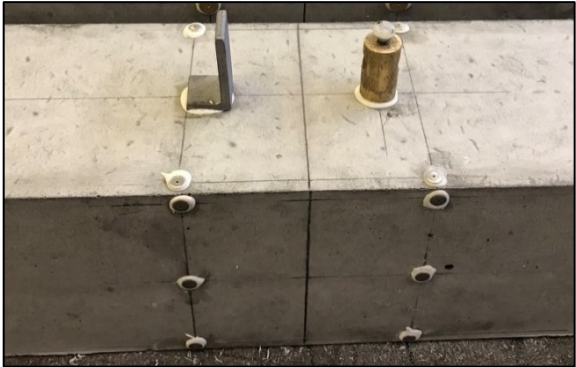
Figure 25: LVDT application in the middle of the specimen
