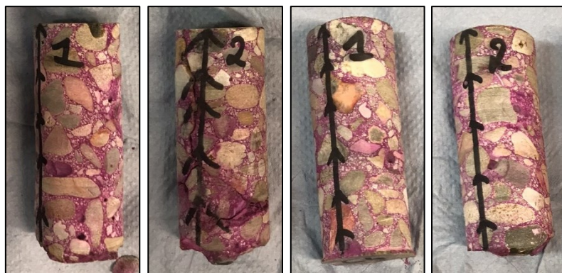
Figure 63: Cores Phenolphthalein test. CN3 cores (on the left), C4 cores (on the right)
