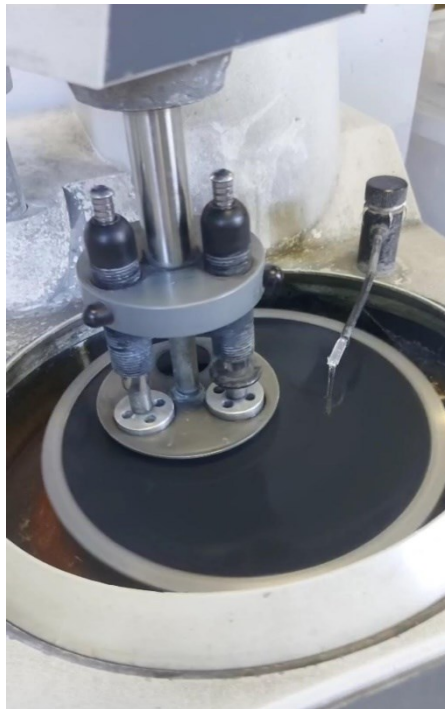
Figure 28: Polishing stage of Titanium samples
