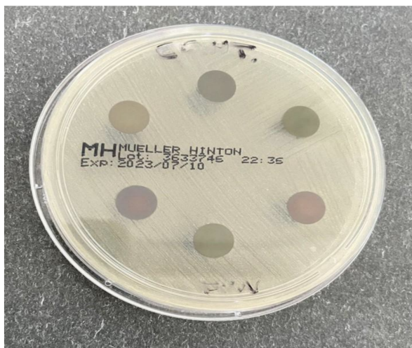
Figure 6.26: Agar plate with samples of control and samples functionalized with GN2-Npm9 peptoid, after incubation of 24 hours at 35°C. There were no differences among the considered specimens, and the absence of halo.
