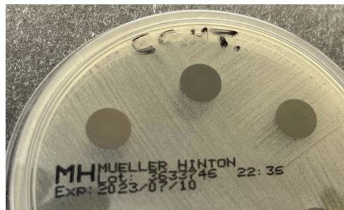
Figure 5.22: Muller Hinton plate with specimens of control tested with S. Epidermidis .
