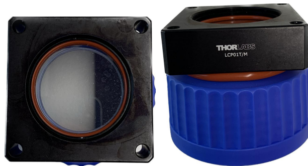
Figure 3.9: Pictures from two different points of view of the sapphire lid, the diameter of the sapphire window is around 5 cm.
