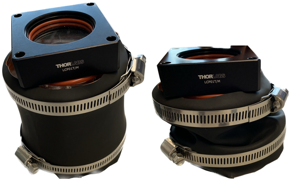
Figure 3.36: On the left the two clamps are concentric, on the right they are displaced.
