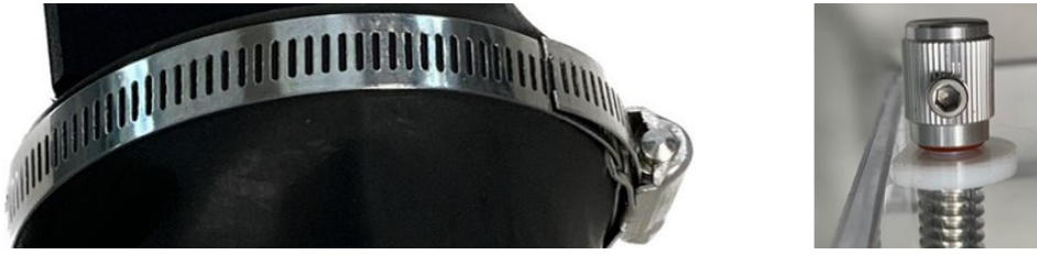
Figure 4.4: On the left, one of the two seals for the membrane. On the right, the seal for the knobs.
