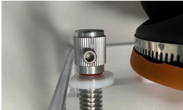
Figure 3.47: On the upper side of the transparent layer, the orange silicon ring. On the other side, the white Teflon ring.
