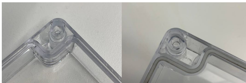
Figure 4.3: On the left, the upper part of the seal as it was purchased. On the right, the same part after the insertion of the silicon layer .
