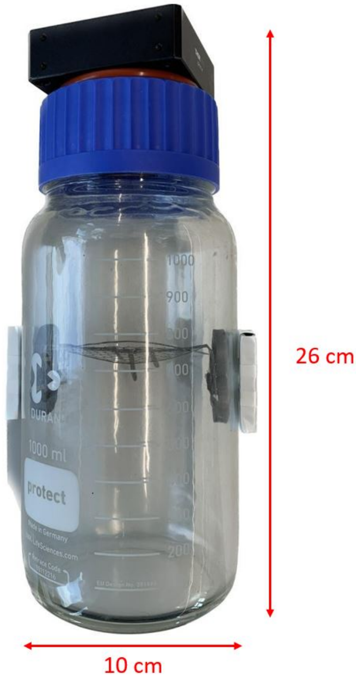
Figure 3.8: Picture of the old container, completely assembled. The total height is about 26 cm and the diameter of the bottle is approximately 10 cm.
