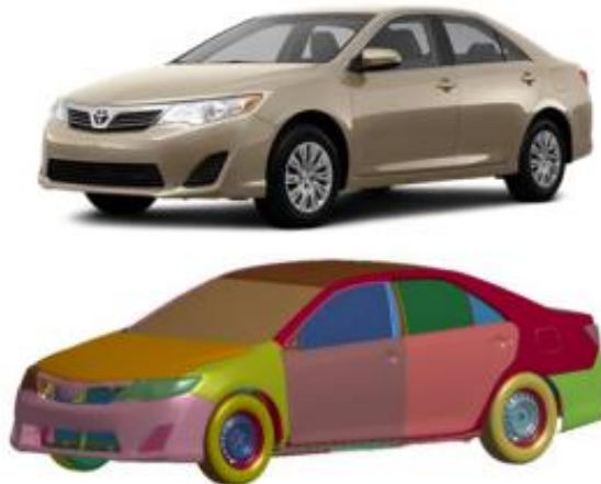
Figura 15 – Toyota Camry Sedan vs Modello FE (CCSA, 2016a)
