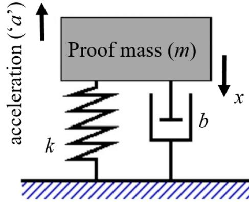
**Figure 3.2:** Dynamic of model of an uni-axial accelerometer. Adapted from [40]
