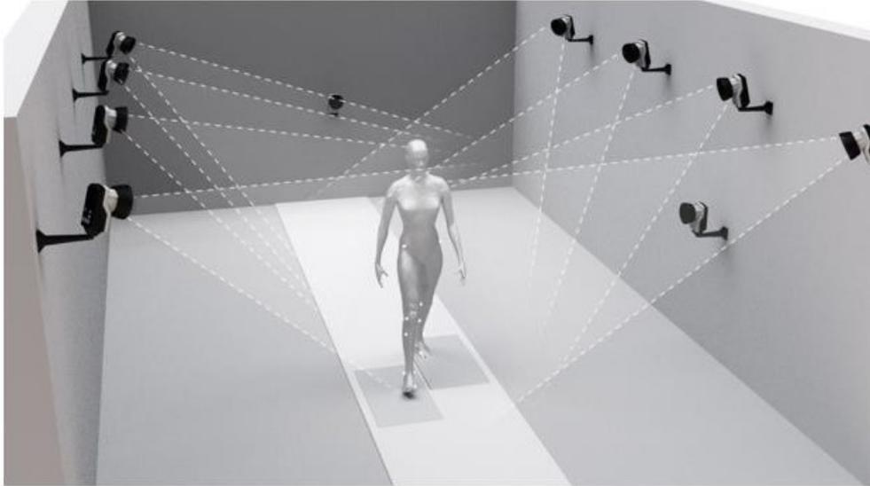
**Figure 3.1:** Illustration of a MOCAP system. Adapted from [37].
