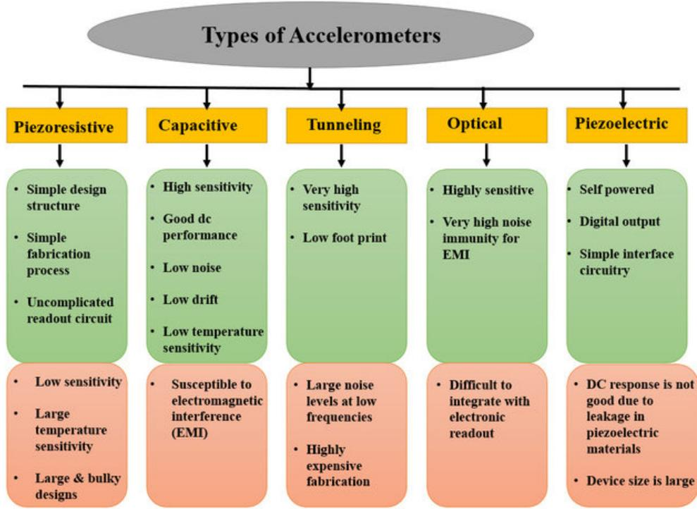
**Figure 3.3:** Advantages and drawbacks of various trasduction schemes. Adapted from [40].
