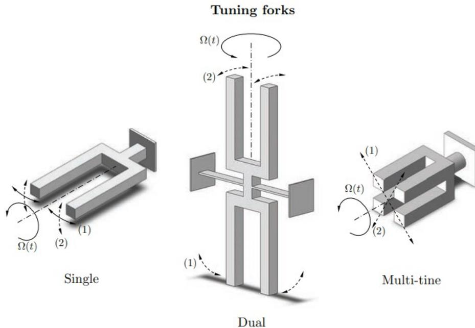
**Figure 3.4:** Common type of vibrating forks gyroscope. From left, single, dual and multi-tine configuration. In figure,  $\Omega(t)$  is the input angular rate, (1) is the primary vibration mode, and (2) is the vibration response due to Coriolis forcing [41].
