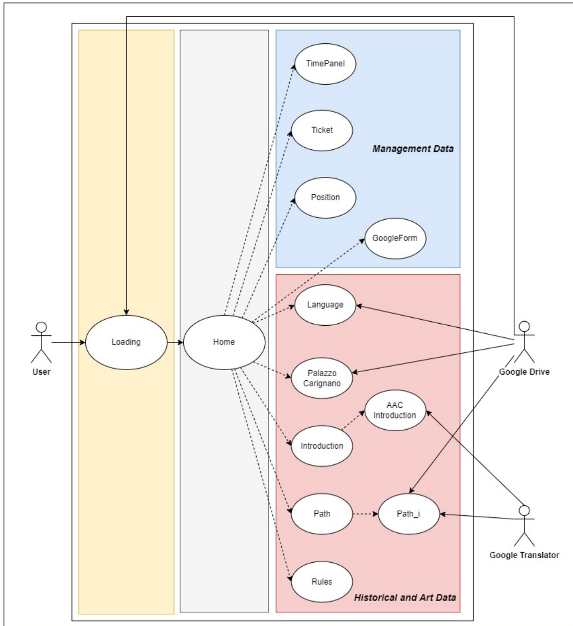
Figure 4.27: The use case diagram shows the actors involved with the system. On the left (human actors) the generic user using the application; on the right (non-human actors) are Google Drive and Google Translator. Also shown are the use cases that characterize the application divided according to the types of data they use.
