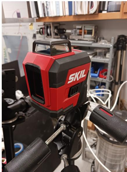
Figure 3.13: SKIL self leveling laser
