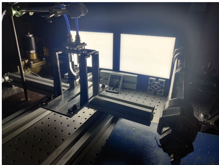
Figure 3.13: Dipropylene glycol test with two LED lamps
