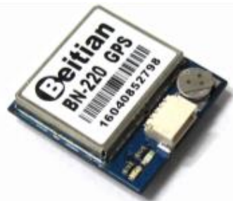
Figure 7: GNSS module (BN-220 GPS Module + Antenna Datasheet)
