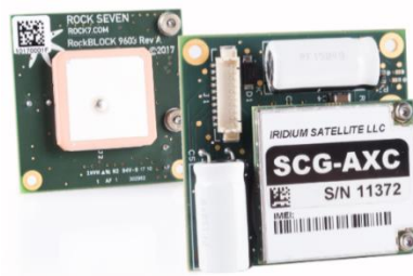
Figure 20: Iridium modem (RockBLOCK 9603 - Datasheet Small, 2023)
