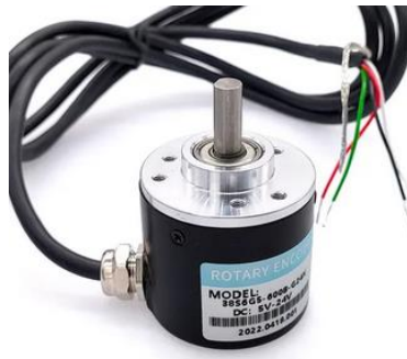
Figure 28: Rotary encoder (38S6G5-B-G24N-Imprimante Incrémentale à Distance, s.d.)
