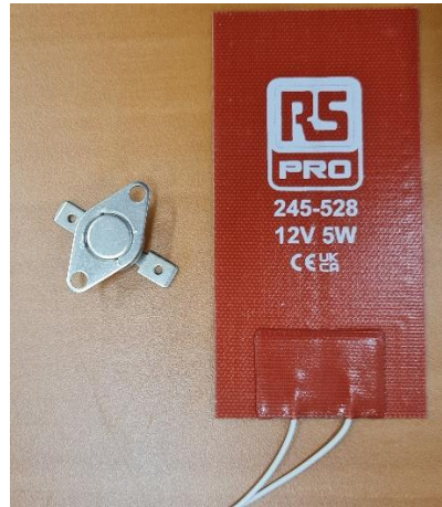
Figure 41: Heater (on the right) and thermal switch (on the left)
