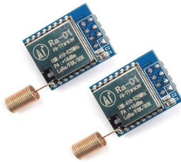
Figure 19: LoRa modems (LoRa SX 1276/77/78/79, 2023)
