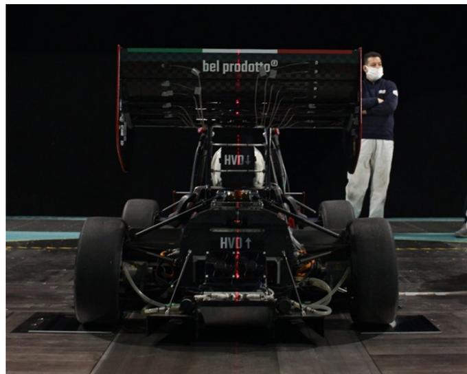
**Figure 4.3:** Pressure taps on the rear wing
