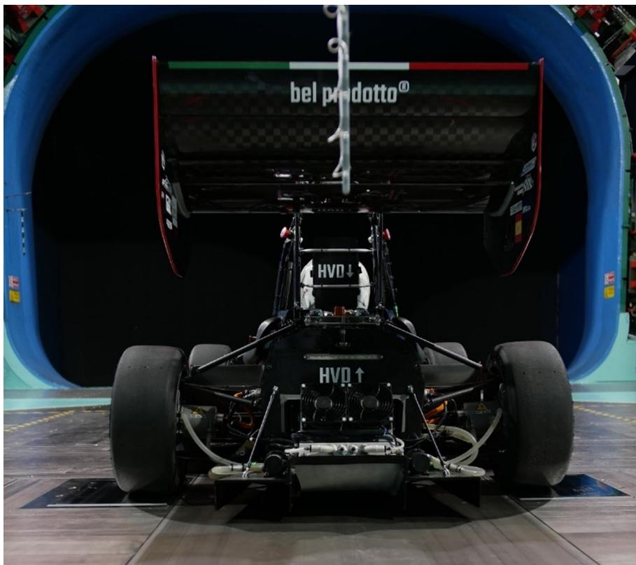
**Figure 4.2:** Car fitting to the Rolling Road Simulation System
