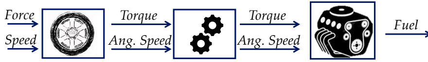
Fig. 5.4 Information flow in a backward kinematic approach [3].
