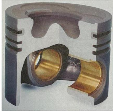
Figure 24. Aluminum piston with a ring carrier in the first groove
