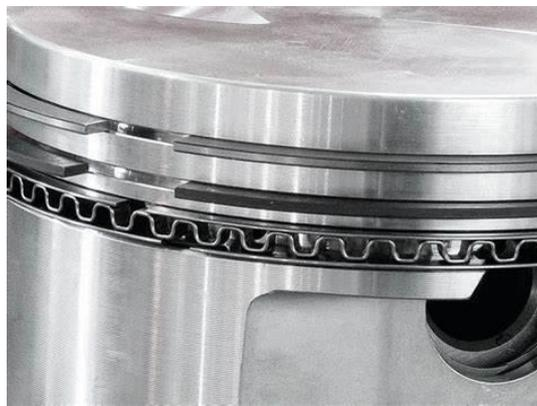
Figure 21. Example of piston rings mounted on a piston
