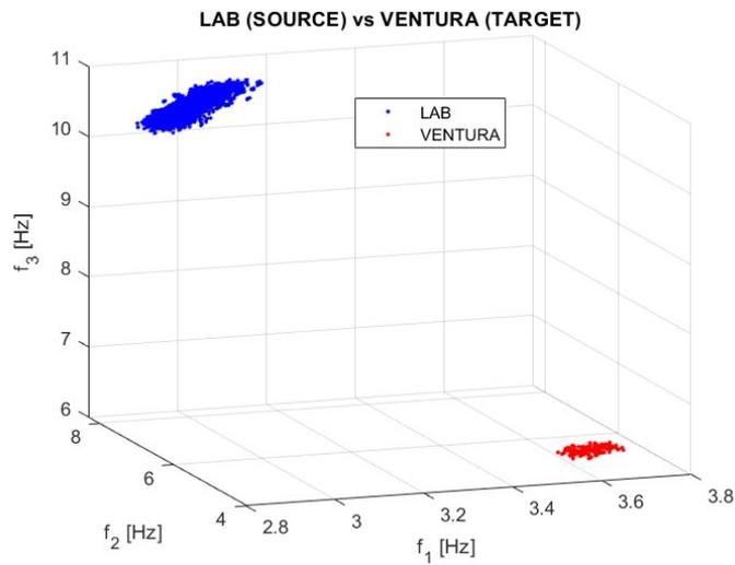
*Figure 51: Natural frequencies 3D plot: analysis II.F.*
