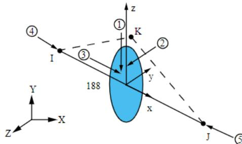
Figure 5: Beam188 element
