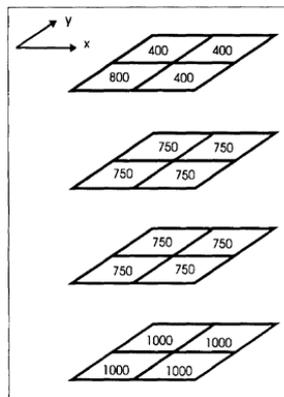
Figure 9: Ventura's Frame added mass [kg]
