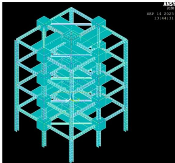
*Figure 13: Unbraced Yellow Frame FEM model*
