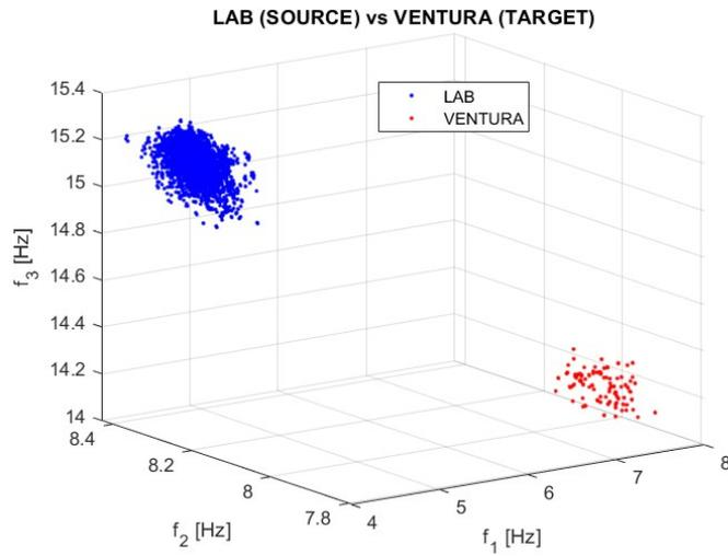
Figure 44: Natural frequencies 3D plot: analysis I.F.
