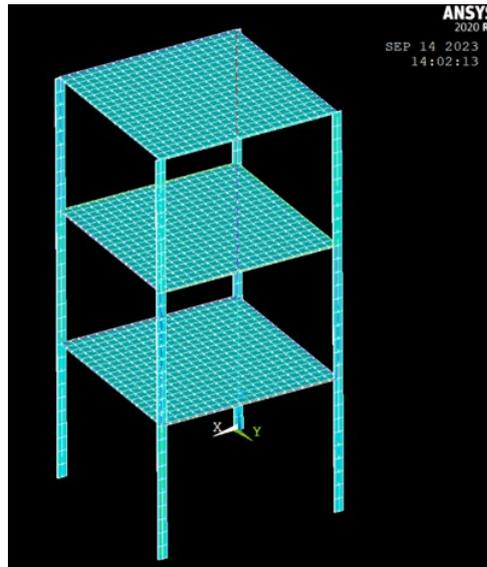
*Figure 17: FEM of the unbraced Laboratory's Frame*
