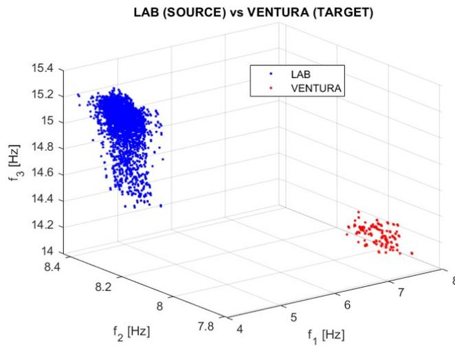
*Figure 43: Natural frequencies 3D plot: analysis I.E.*
