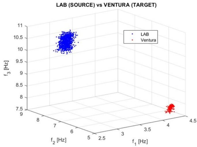
Figure 46: Natural frequencies 3D plot: analysis II.A.
