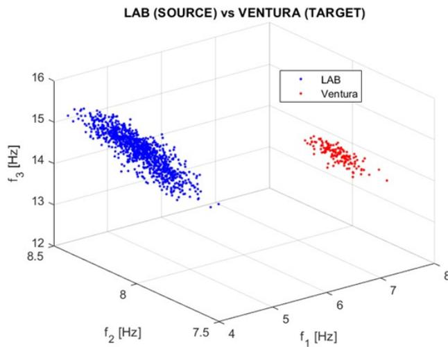
Figure 39: Natural frequencies 3D plot: analysis I.A.
