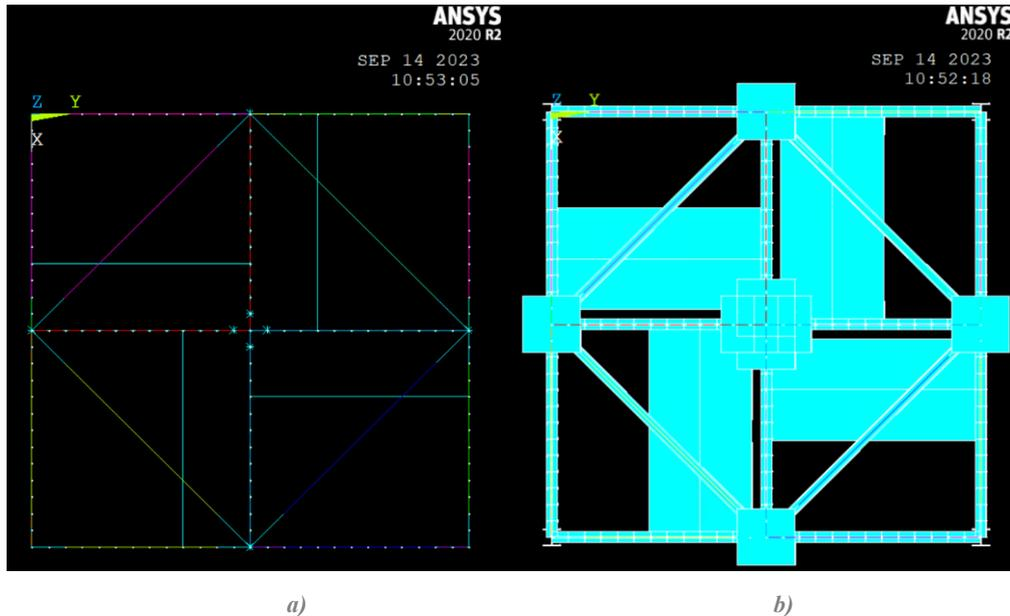
Figure 10: Steel frame plan view: a) elements and nodes for applied mass; b) meshed elements
