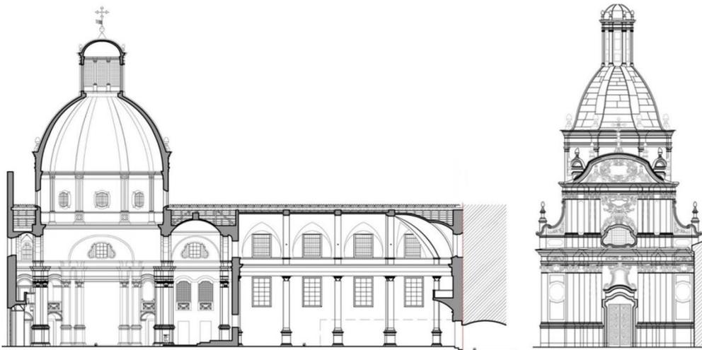
Figure 32: Longitudinal section (left) and Front view (right) of Santa Caterina's Church drawings (Ceravolo, Lenticchia, Miraglia, & Scussolini)
