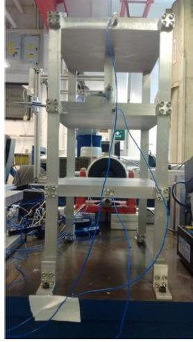
Figure 16: Experimental shear-structures (Gardner, Bull, Dervilis, & Worden, 2022)
