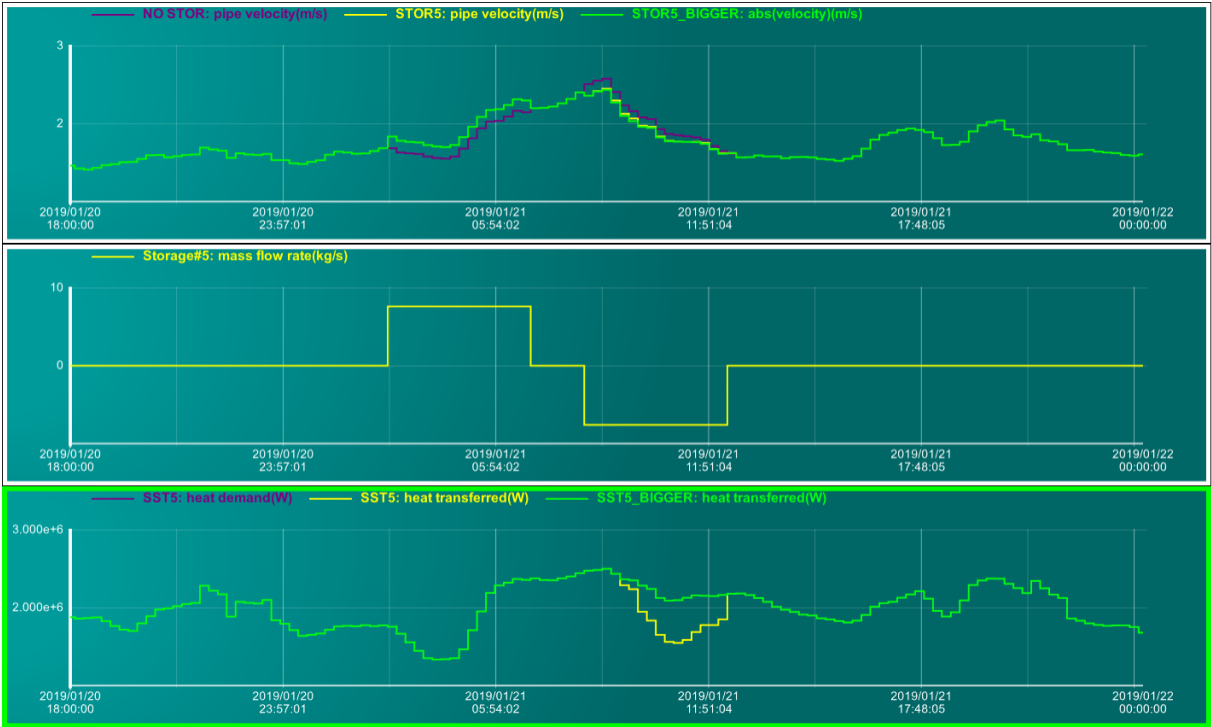
Figure 21. New simulation: Profile of the velocity [m/s] in the most critical pipe; Mass flow rate [kg/s] inside the storage; Heat Demand-Heat Transferred [W].
