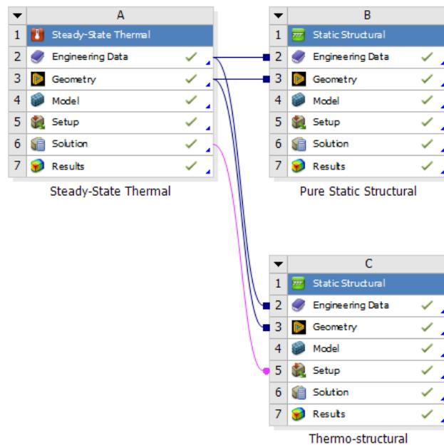
Figure 46 Setting up a thermo-structural analysis in ANSYS
