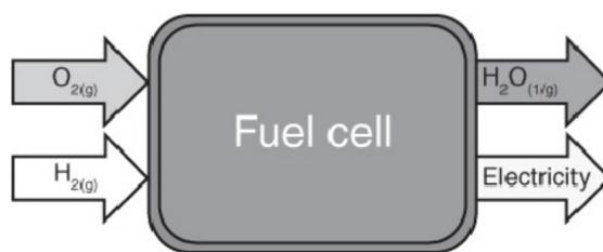
**Figure 1.11:** Fuel cell reactants and products[6]
