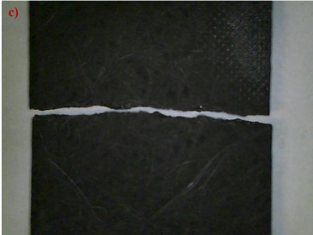
*Figure 60: Microscopic image of 0° fractured specimen near the grip*
