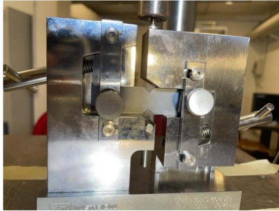
*Figure 22: Shear testing configuration*
