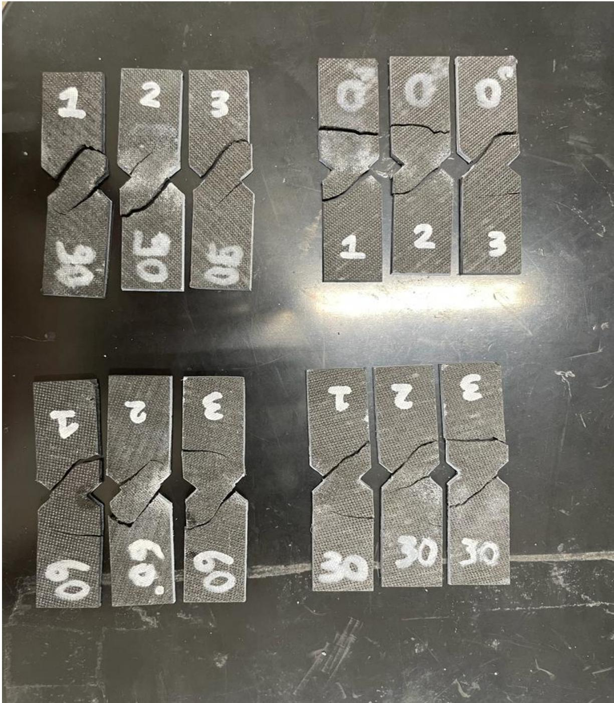
Figure 51: Specimens after shear test
