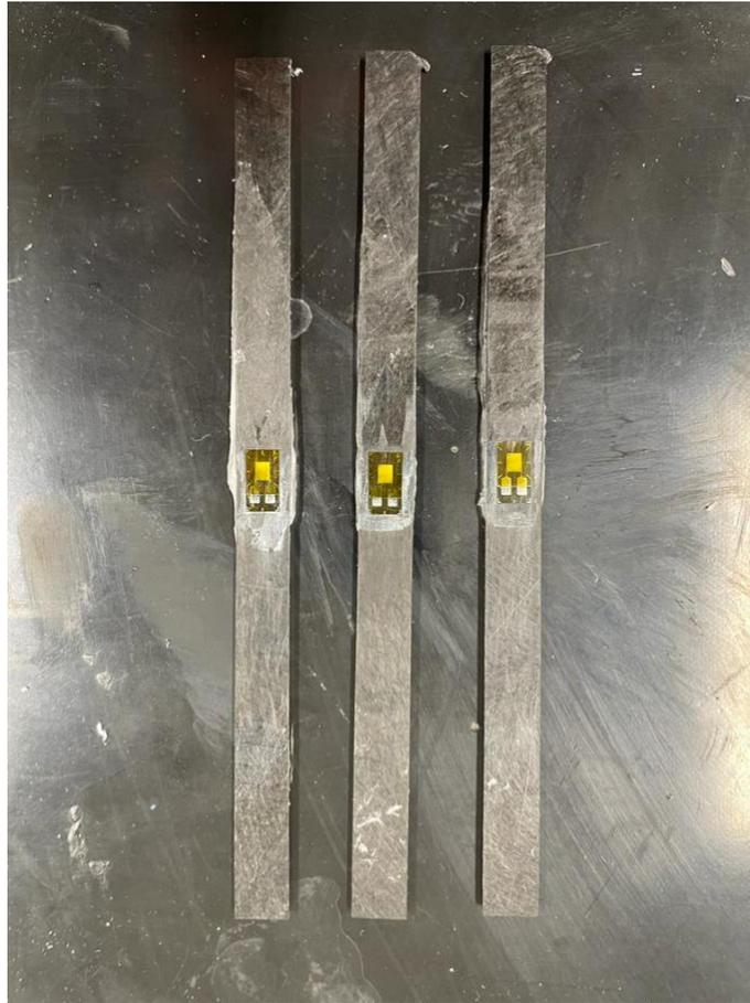
*Figure 17: Strain gauges bonded to compression specimens.*
