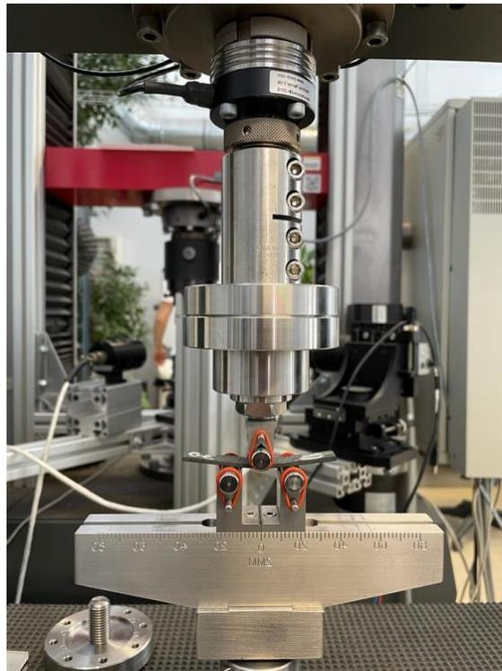
*Figure 18: Specimen undergoing bending during three-point bending test.*
