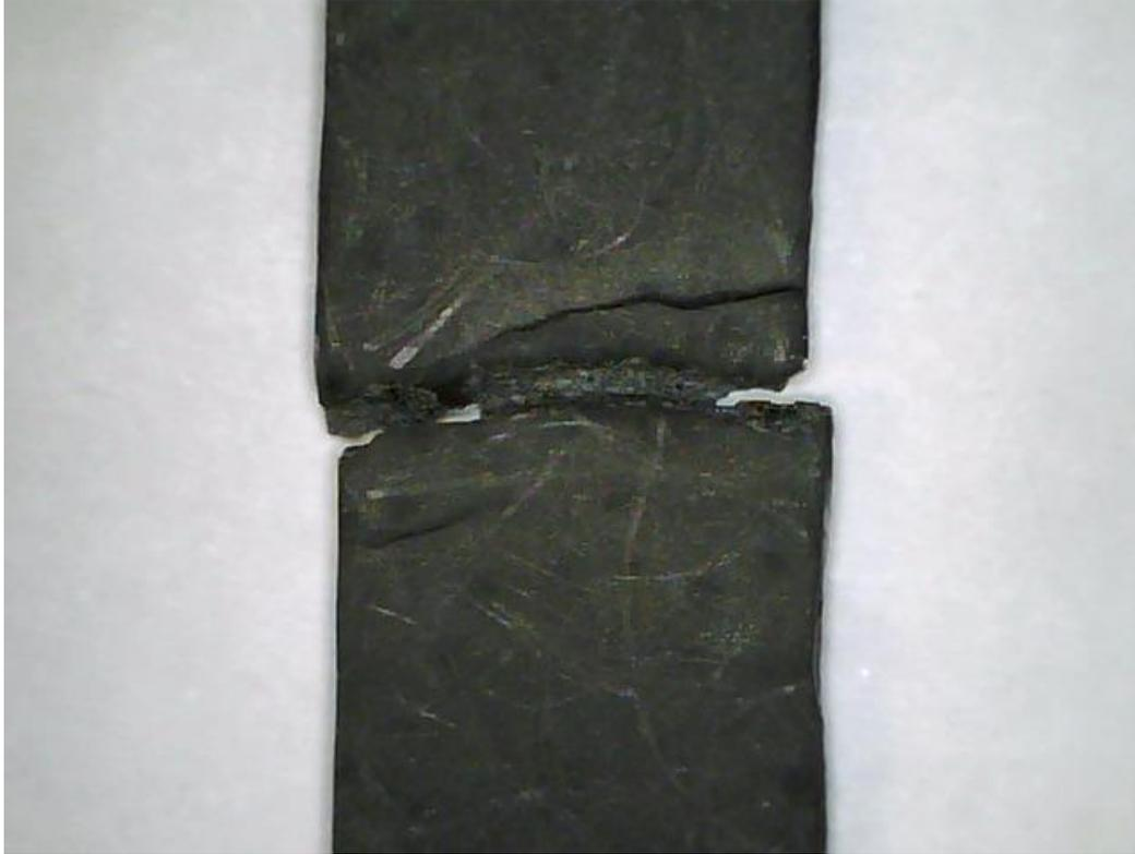
*Figure 68: Microscopic image of 90° fractured specimen*
