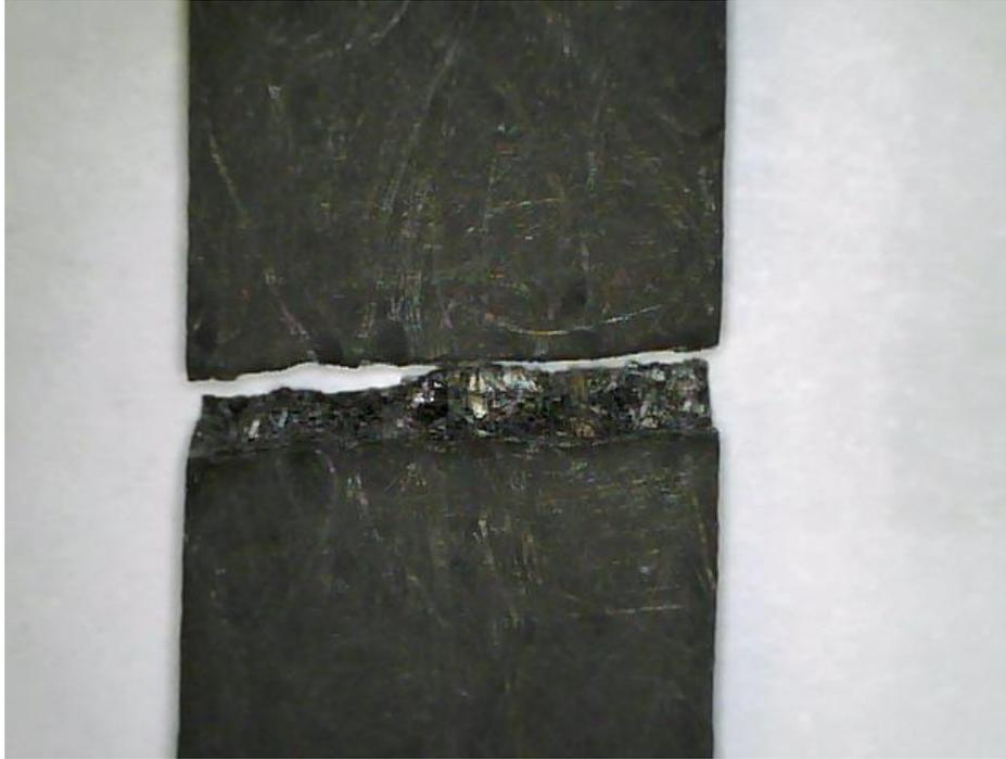
*Figure 58: Microscopic image of 90° fractured specimen*
