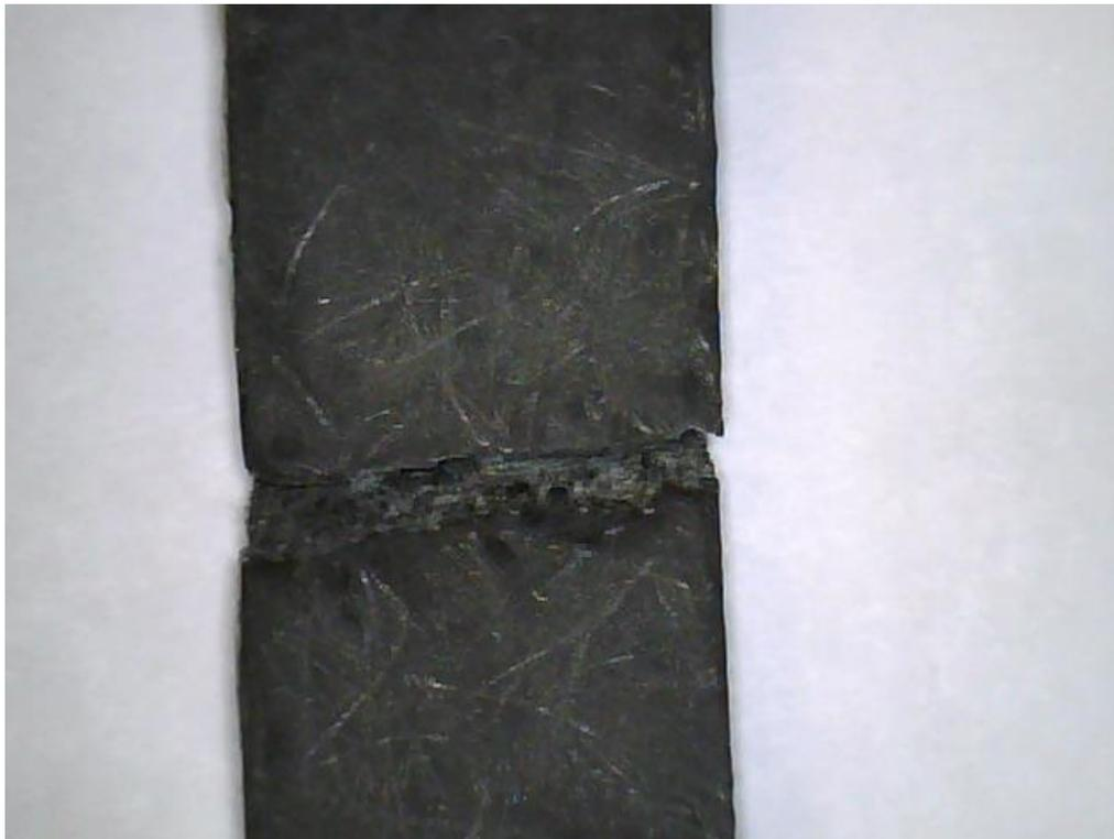
*Figure 67: Microscopic image of 60° fractured specimen*
