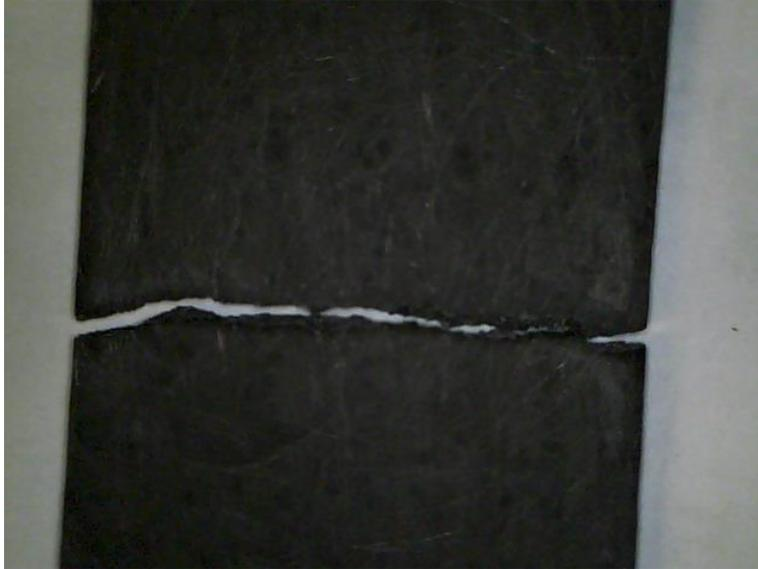
*Figure 63: Microscopic image of 90° fractured specimen*
