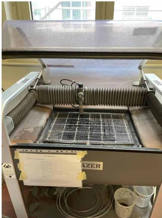
*Figure 10: Water jet cutting machine.*
